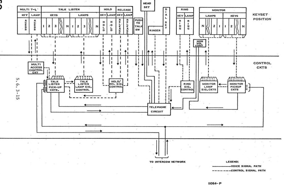
Figure 5.6-9 Intercom Station Block Schematic
