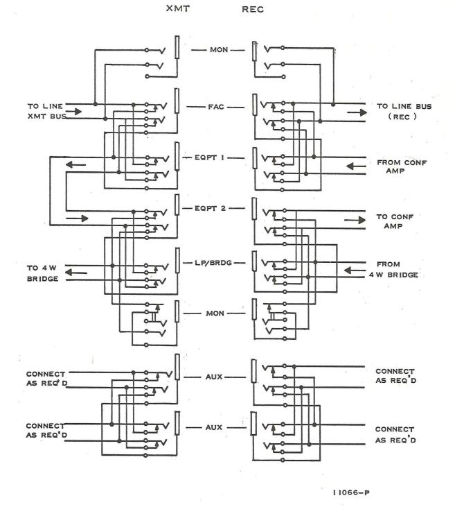
Figure 5.6-11 Typical Universal Jack Circuit
