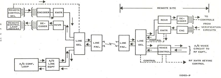
Figure 5.6-10 A/G Control System Block Diagram
