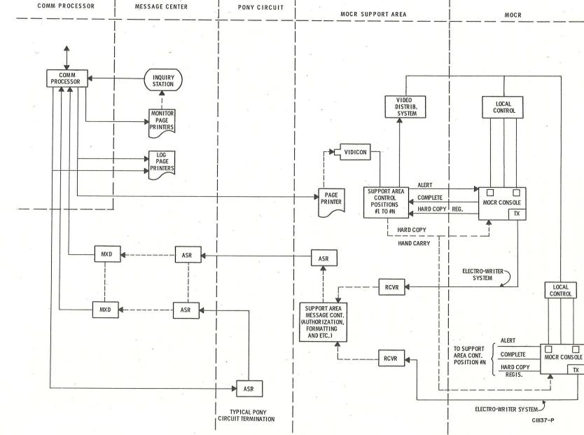
Figure 5.6-5 Recommended Configuration for Pony Circuit Message Delivery
