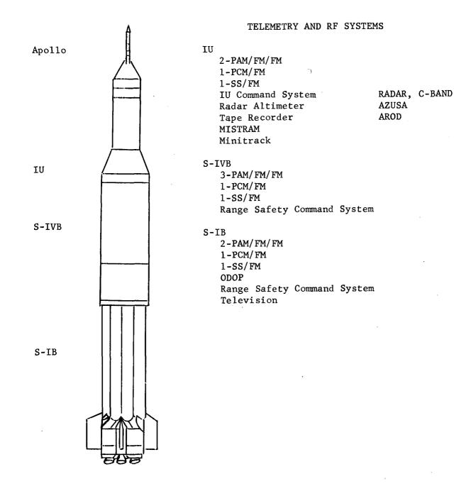
FIGURE 4. SATURN IB (R&D) INSTRUMENTATION SYSTEMS.
