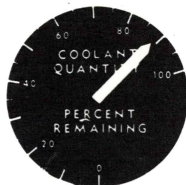
COOLANT QUANTITY INDICATOR
