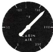
CABIN TEMPERATURE INDICATOR
