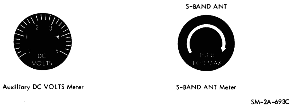
Figure 4-10. Telecommunication System Meters
