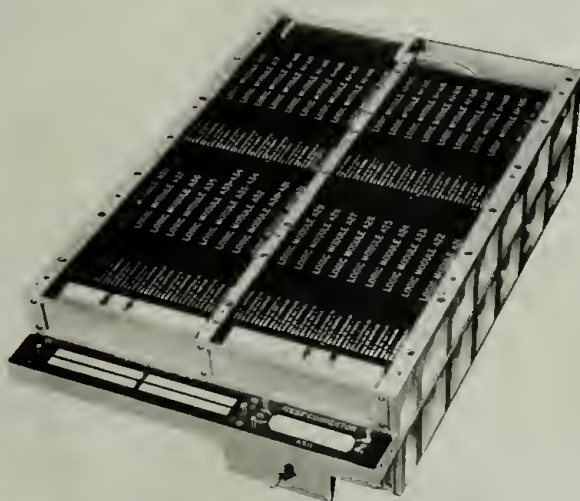
Figure 3-8. Logic Tray A
