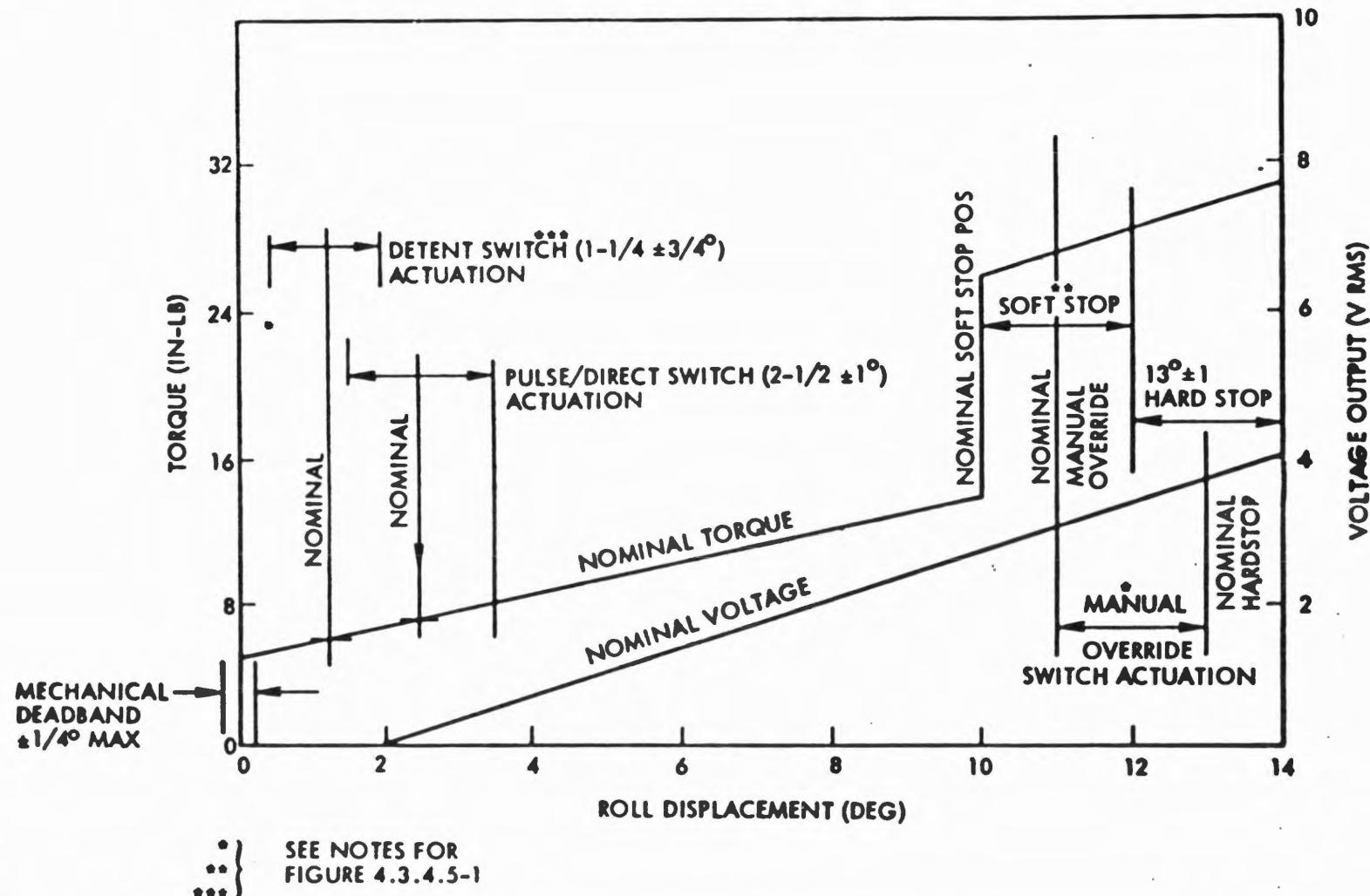
Figure 4.3.4.5-2. Torque and Voltage Output versus Roll Displacement
