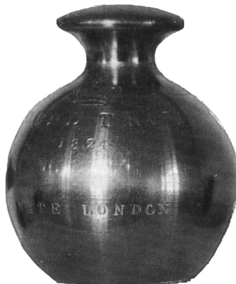
Figure 2.4: The troy pound of the U.S. Mint, basis for all U.S. weights from 1828 to 1911
