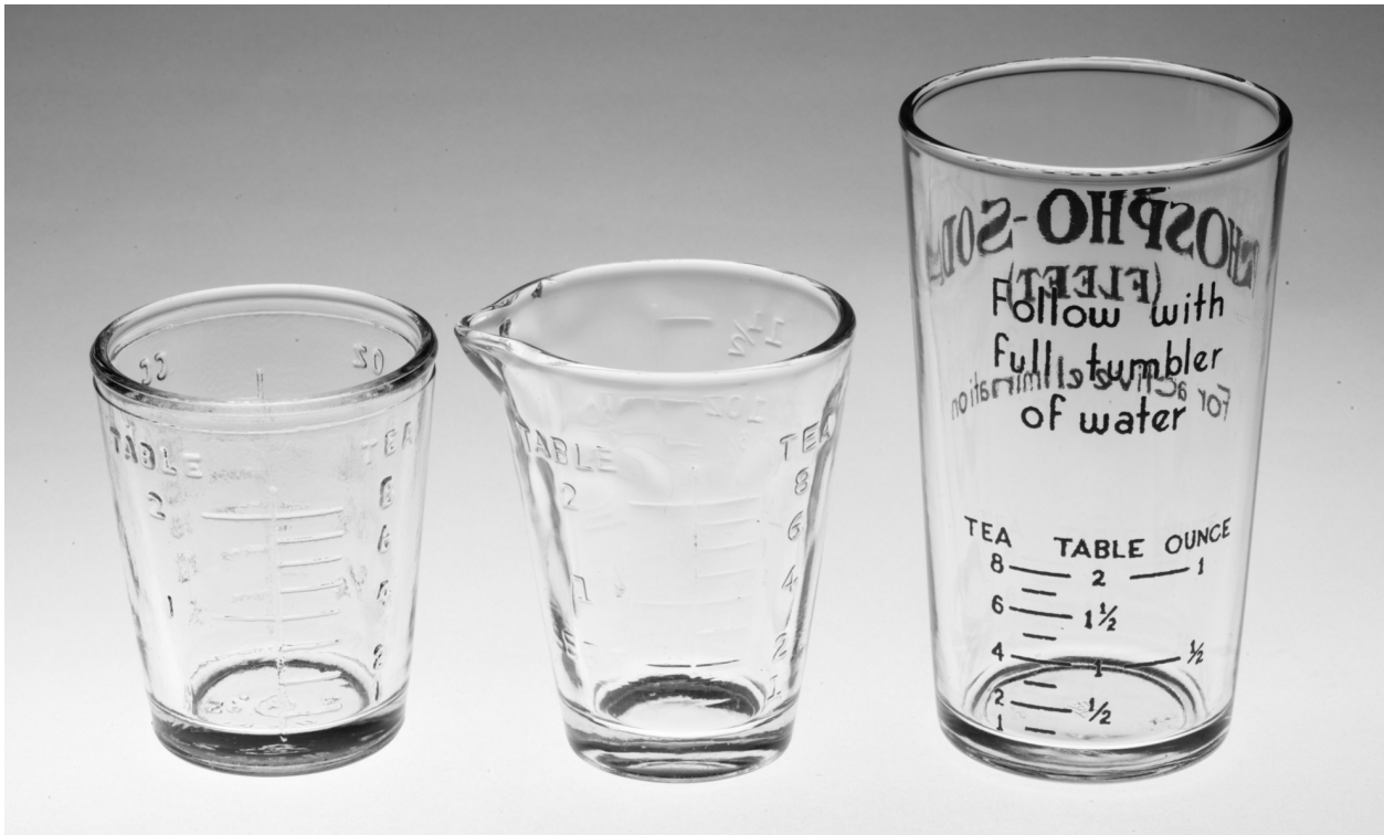
Figure 3.2: Early 20th century American glass medicine cups showing former definition of the teaspoon as a quarter of a tablespoon, equivalent to the fluid dram ( \frac{1}{8} fluid ounce). The teaspoon is now defined in the U.S. as a third of a tablespoon ( \frac{1}{6} fluid ounce)
