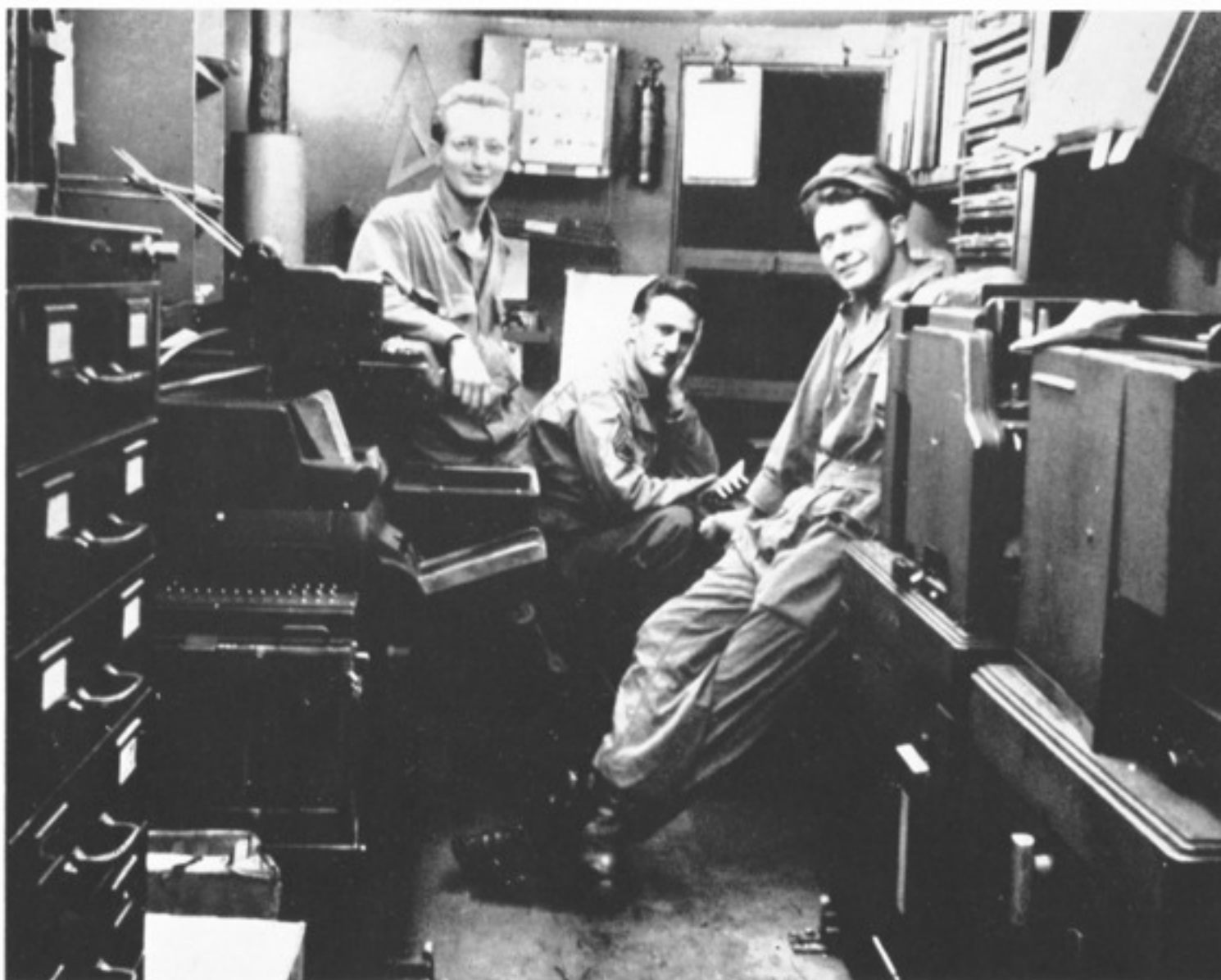
The inside of a machine trailer. Euth is leaning on a tabulator. We had three, one in each machine trailer. Griffis is sitting at a key punch. There were four of these, one in each machine trailer and one in the administration trailer. Johnson is leaning on one of the three collators. In the right foreground is one of the three interpreters. Not shown are the six sorters, located two to each machine trailer.
