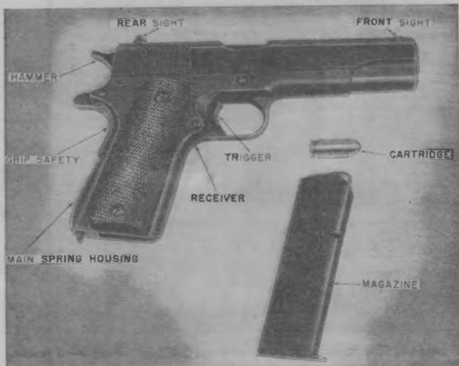
Figure 66. The automatic pistol, caliber .45. Weight (with magazine)—2.44 pounds. Recoil-operated, magazine-fed. Maximum effective range—1,640 yards.
