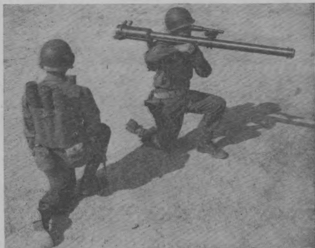
Figure 73. The 57-mm. recoilless rifle, M18. Weight—45 pounds; weight with tripod—98 pounds. Weight of projectile—2¾ pounds. Range—4,340 yards.
