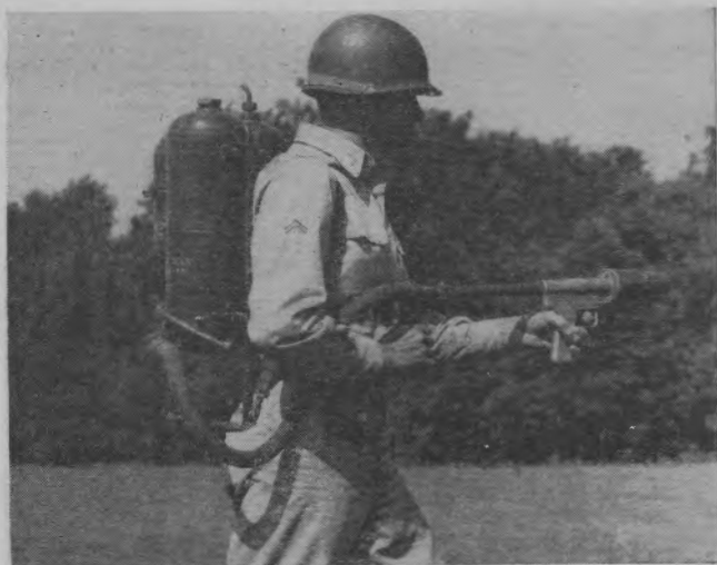
Figure 77. The portable flame thrower, M2-2. Weight—68 to 72 pounds. Range—40 yards.
