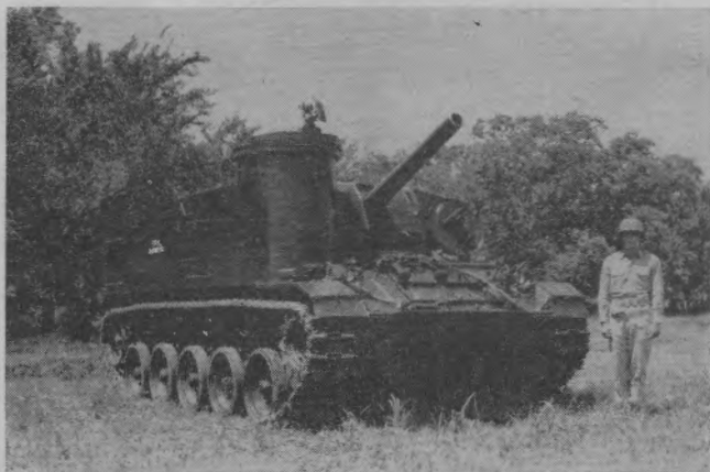
Figure 88. 105-mm. howitzer, M4, on motor carriage, M37. Weight—46,000 pounds. Weight of projectile—33 pounds. Range—12,205 yards. Rate of fire—4 rounds per minute.
