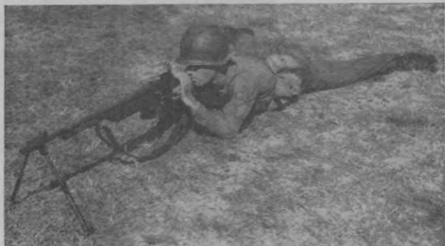
Figure 67. The Browning automatic rifle, caliber .30, M1918A2. Weight—19.5 pounds. Range—3,500 yards. Maximum rate of fire—350 to 550 rounds per minute.
