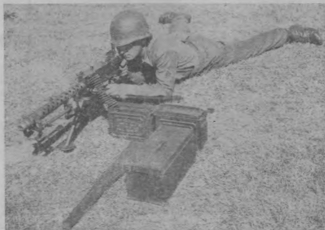
Figure 71. The Browning machine gun, caliber .30, M1919A6 (light). Weight—49.75 pounds. Range—3,500 yards. Maximum rate of fire—400 to 550 rounds per minute.
