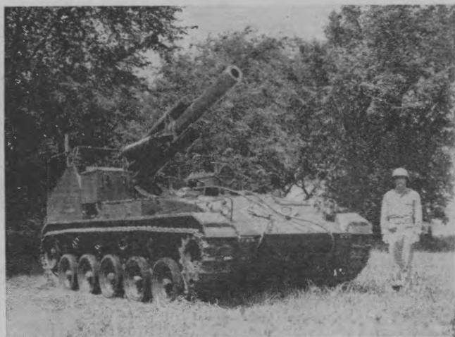
Figure 91. The 155-mm. howitzer, M1, on motor carriage, M41. Weight—42,500 pounds. Weight of projectile—95 pounds. Range—16,355 yards. Rate of fire—2 rounds per minute.
