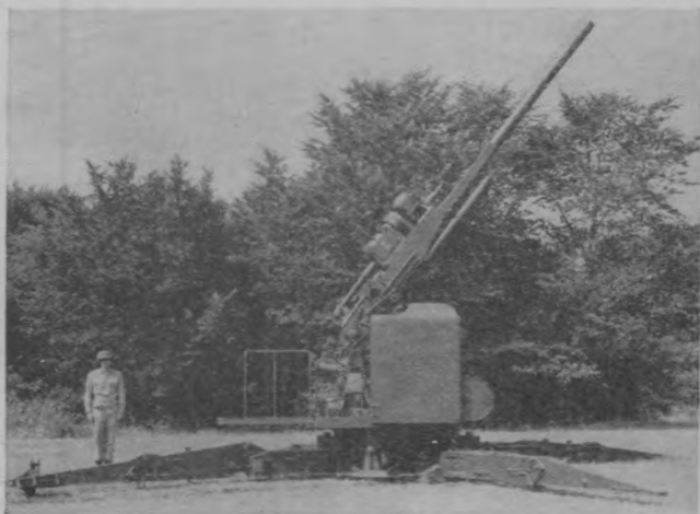
Figure 86. The 90-mm. gun, M2, on anti-aircraft mount, M2. Weight—25,850 pounds; weight with wheels—32,300 pounds. Weight of projectile—24 pounds. Vertical range—11,800 yards. Horizontal range—19,560 yards. Rate of fire—23 to 28 rounds per minute.
