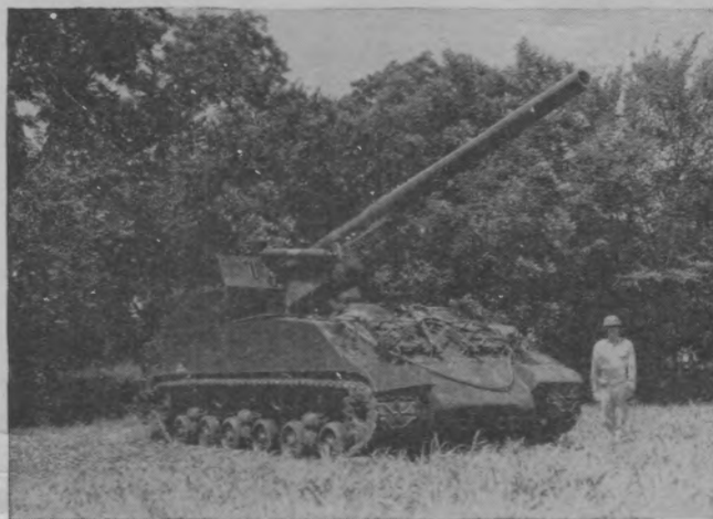
Figure 93. The 155-mm. gun, M2, on motor carriage, M40. Weight—81,000 pounds. Weight of projectile—95 pounds. Range—25,715 yards. Rate of fire—2 rounds per minute.
