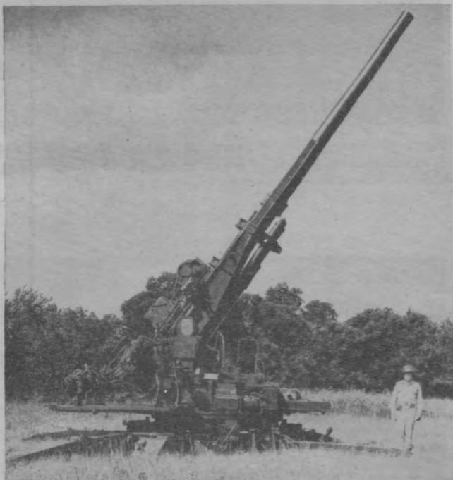
Figure 89. The 120-mm. gun, M1, on anti-aircraft mount, M1A1. Weight—48,000 pounds; weight with wheels—61,500 pounds. Weight of projectile—50 pounds. Vertical range—15,500 yards. Horizontal range—27,162 yards. Rate of fire—10 to 15 rounds per minute.
