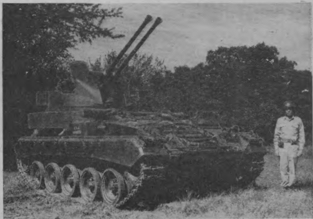
Figure 84. The 40-mm. gun (twin), M2, on motor carriage, M19. Weight—41,165 pounds. Weight of projectile—2 pounds. Vertical range—7,627 yards. Horizontal range—10,850 yards. Rate of fire—240 rounds per minute.
