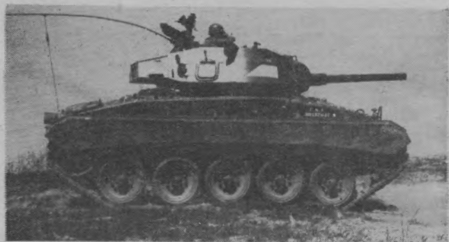
Figure 98. The light tank, M24 (General Chaffee). Weight—20 tons. Caliber of gun—75-mm. Range of gun—8,890 yards. Speed—34 mph.
