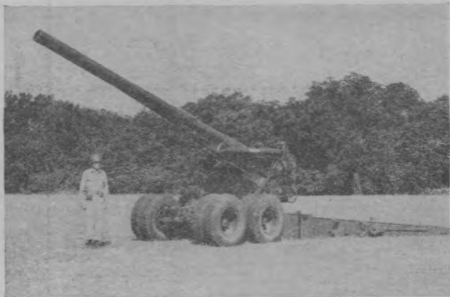
Figure 92. The 155-mm. gun, M2, carriage, M1. Weight—27,700 pounds. Weight of projectile—95 pounds. Range—25,715 yards. Rate of fire—2 rounds per minute.
