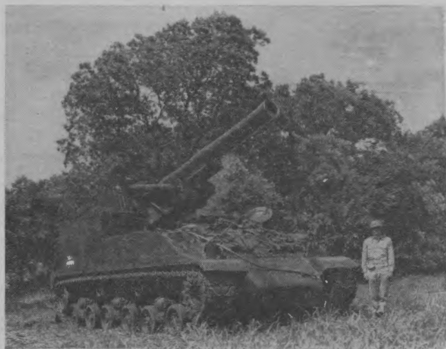
Figure 95. The 8-inch howitzer, M2, on motor carriage, M43. Weight—80,000 pounds. Weight of projectile—200 pounds. Range—18,510 yards. Rate of fire—3 rounds every 2 minutes.
