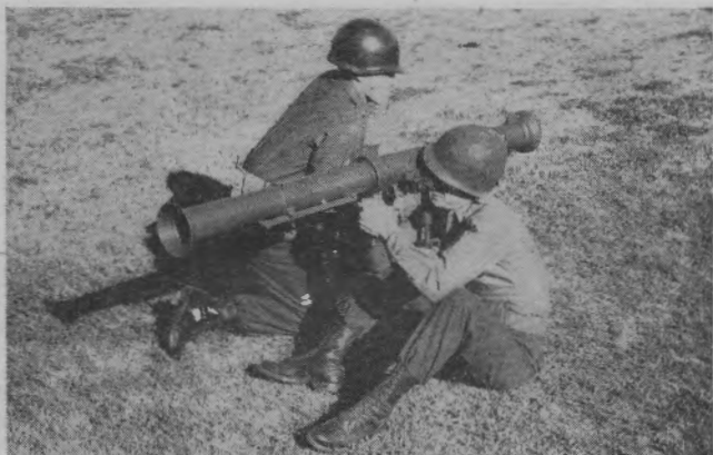
Figure 76. The 3.5-inch rocket launcher, M20. Weight—15 pounds. Weight of projectile—8.5 pounds. Range—960 yards.
