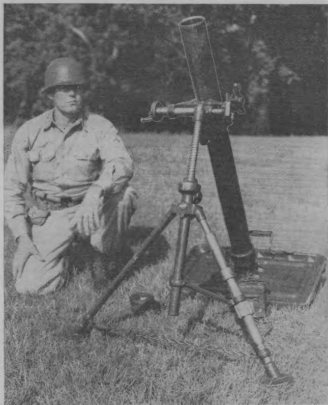
Figure 80. The 81-mm. mortar, M1. Weight—136.5 pounds. Range—3,290 yards. Weight of projectile—7 to 13 pounds. Rate of fire—30 to 35 rounds per minute.
