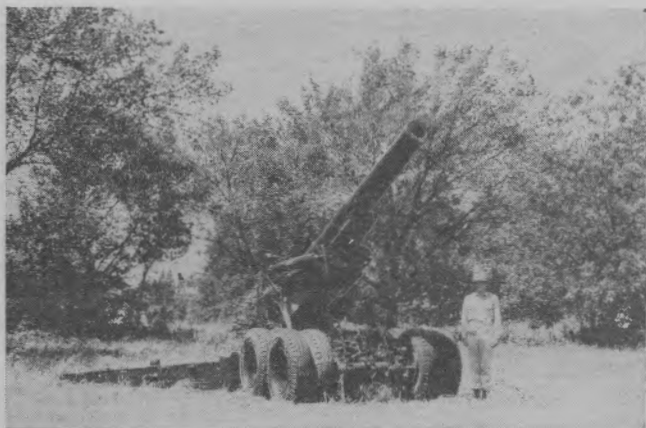
Figure 94. The 8-inch howitzer, M2, on carriage, M1. Weight—28,000 pounds. Weight of projectile—200 pounds. Range—18,510 yards. Rate of fire—3 rounds every 2 minutes.
