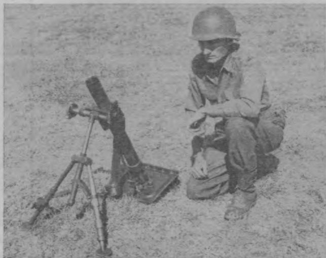
Figure 79. The 60-mm. mortar, M19. Weight—45.2 pounds. Weight of projectile—3 to 4 pounds. Range—1,985 yards. Rate of fire—30 to 35 rounds per minute.
