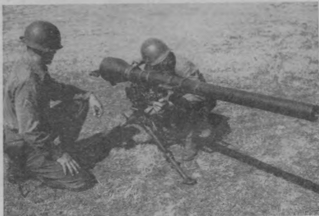
Figure 74. The 75-mm. recoilless rifle, M20. Weight—115 pounds; weight with tripod—168 pounds. Weight of projectile—14 pounds. Range—7,200 yards.
