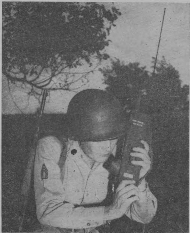
Figure 53. The "walkie talkie." Type of transmission—voice. Range—1 mile. Used by—infantry squads and platoons, and artillery forward observers.
