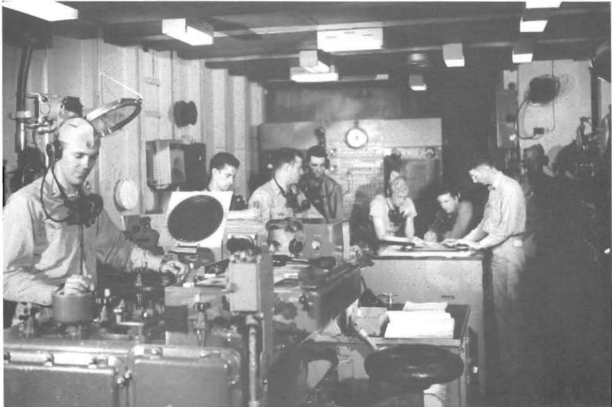
One of MISSOURI's two main-battery plotting rooms. Here, many inputs are combined to produce continuous train and elevation orders to the guns. (See p. 164.)
