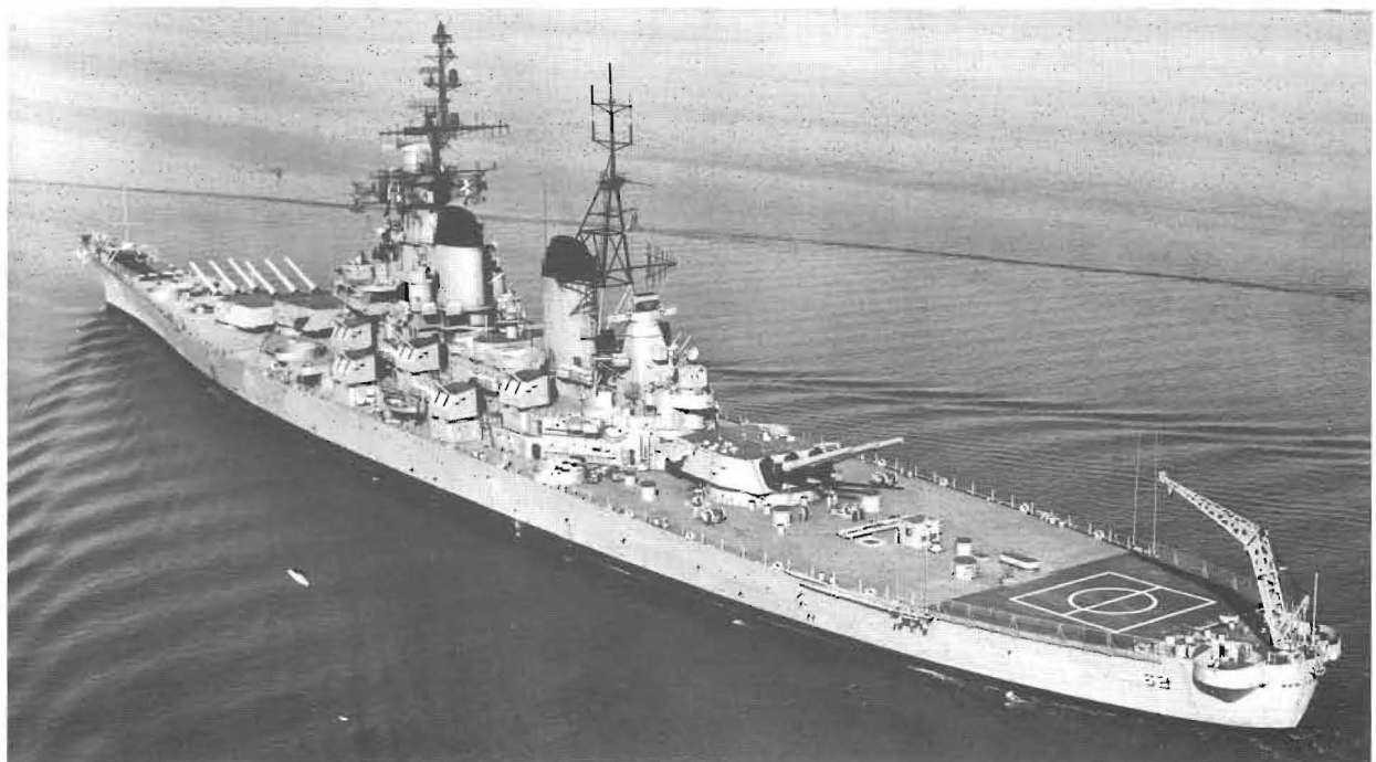
NEW JERSEY prepares for Vietnam, April 1968 after an austere reactivation. 40mm guns are gone, and her new electronic suit includes an ECM installation for antimissile defense.
