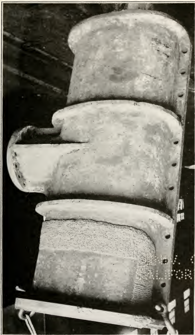
S. S. SANYOS: SECOND I. P. VALVE CHEST AFTER WELDING AT NAVY YARD, PHILADELPHIA, PA.
