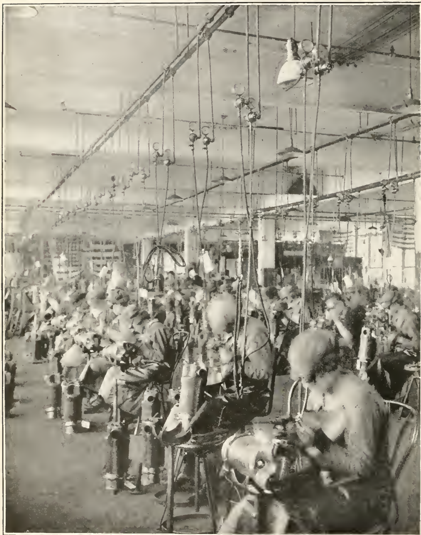
WELDING WATER JACKETS OF LIBERTY ENGINES, PACKARD COMPANY.
