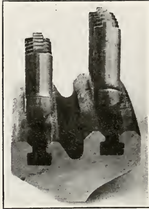
TURBINE BLADING, BETHLEHEM CORPORATION.
