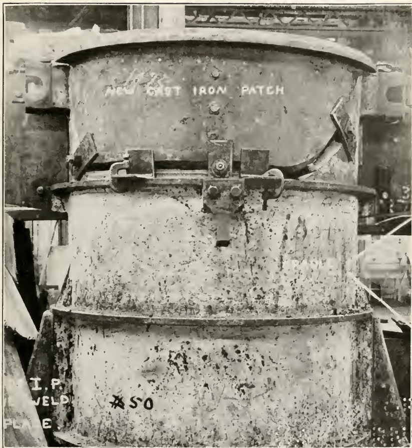
S. S. NECKAR, 2D I. P. CYLINDER; CAST IRON PATCH READY FOR WELDING.
