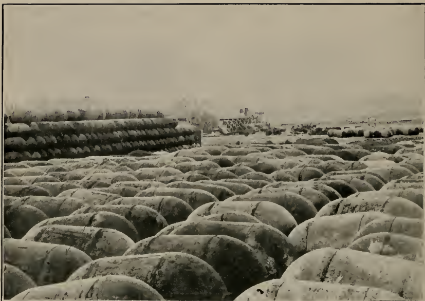
Sphero-cylindrical steel buoys stowed at Carness Point. These buoys were used for marker buoys for the mine fields. (Page 68.)
