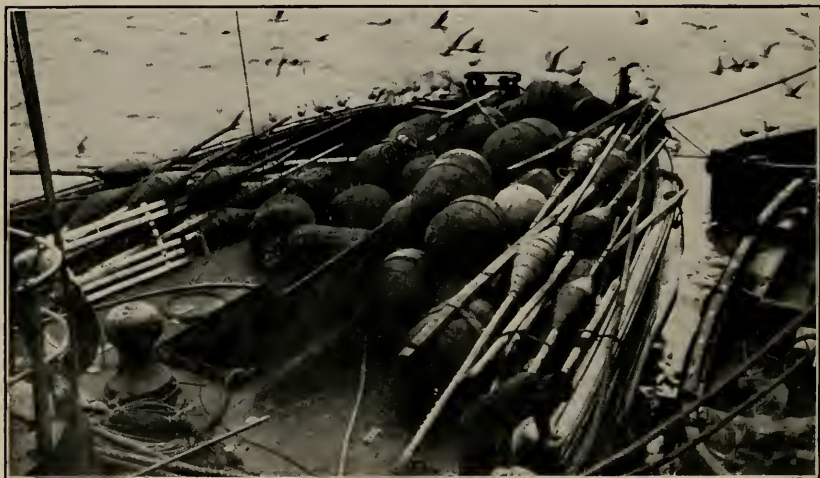
A deckload of marker buoys and dan buoys. The long slender spars with a barrel in the middle are called dan buoys. (Page 68.)
