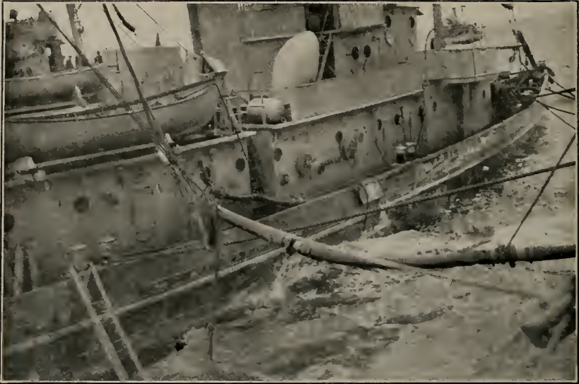
U. S. S. Pelican shortly after she was countermined, showing the pump line from U. S. S. Eider keeping the Pelican afloat. (Page 41.)
