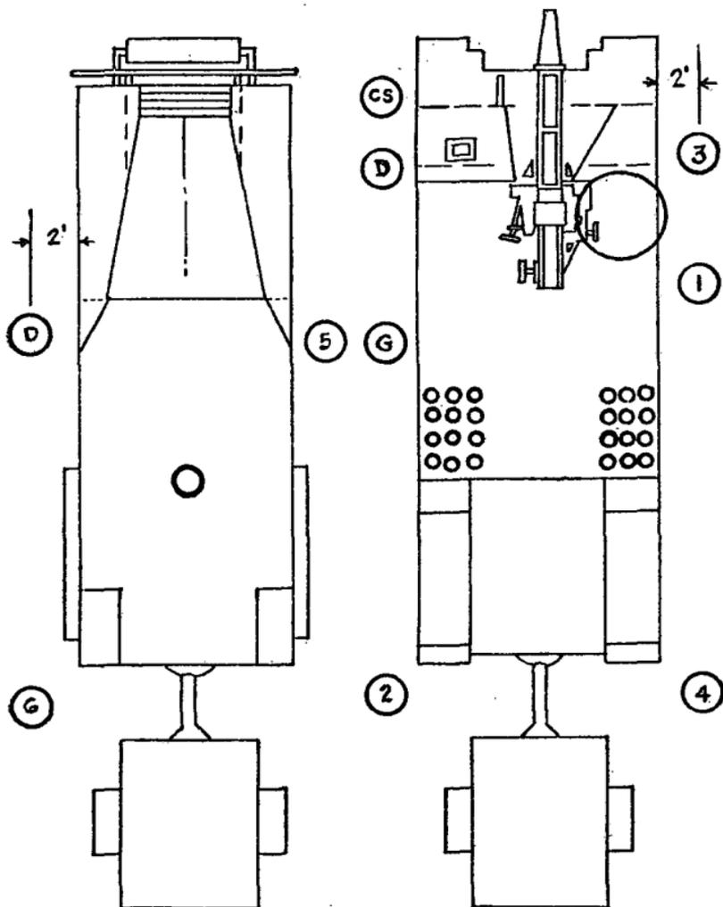
FIGURE 5.—Posts of section, dismantled, 105-mm howitzer motor carriage M-7. (Note that in mounting the driver precedes the chief of section and No. 1 precedes No. 3.)
