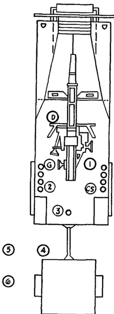
FIGURE 8.—Post of cannoneers prepared for action, 105-mm motor carriage T-19. (The ammunition carrier is placed for perimeter defense and the driver mans the caliber .30 machine gun.)
