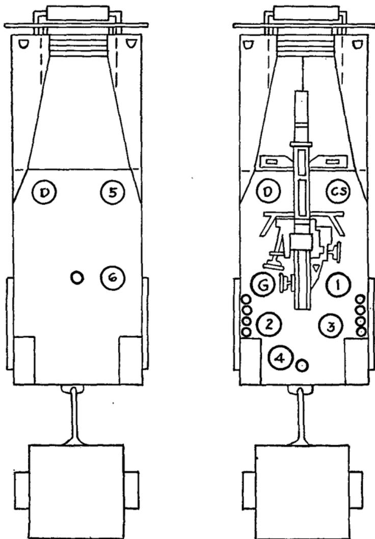
FIGURE 6.—Posts of section, mounted, 105-mm howitzer motor carriage T-19.
