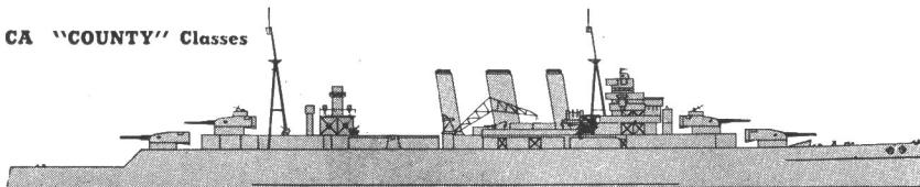
KENT Class—CUMBERLAND and SUFFOLK have hull broken aft. Balance of Class flush-deckers, with same general rig as DEVONSHIRE. Hangar removed from CUMBERLAND
