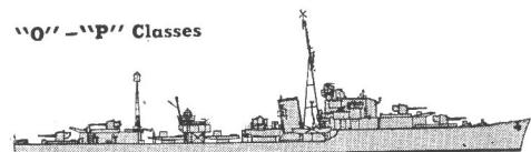
First of the new fleet destroyers which combined the one-stack "J" arrangement with the armament plan of the "A" to "I" series. 1941-42.
