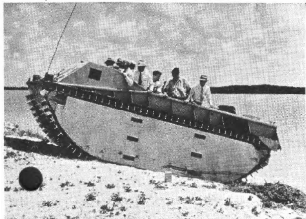
▼ LVT(1)—Tracked landing vehicle, unarmoured.
