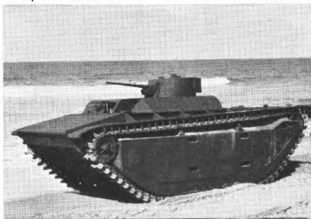
▼ LVT(A)1—Tracked landing vehicle, armoured.
