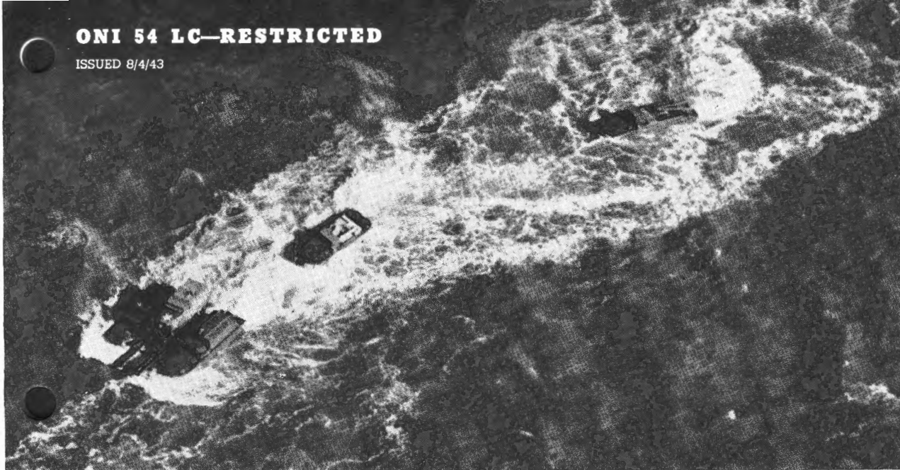
▼ LVT(1)—Tracked landing vehicle, unarmoured.
