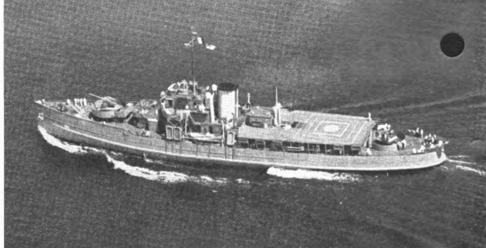
◆ COBB—Ex-passenger vessel converted to base helicopters in convoy work
