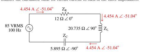
Now we have all the information needed to calculate voltage drop across each of the passive components, using Ohm's Law:
