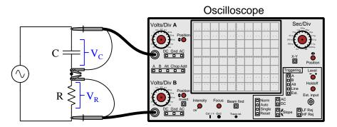
Given that the two channels' ground clips are electrically common to each other, we can actually eliminate either one of them and still have the same result:
