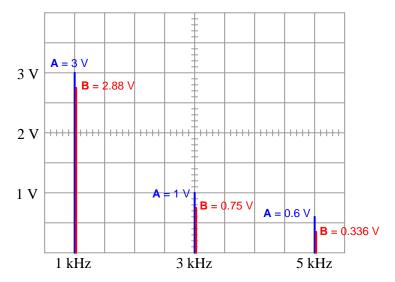
The relative peak heights of the channel A signal (3 Volts, 1 Volt, 0.6 Volts) are simply the result of the Fourier series for a square wave and has nothing to do with the RC network. The ratios between peak heights of channel A and channel B at each harmonic frequency, however, are unique to the 4.7 k $\Omega$  and 0.01  $\mu$ F RC network because those voltage pairs represent the attenuation of this particular network at each of those sinusoidal frequencies.
