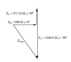
Since these stacked vectors comprise a right-triangle, we may calculate total impedance  $(Z_{total})$  magnitude using the Pythagorean Theorem with just the magnitudes  $^{10}$  of  $Z_R$ ,  $Z_L$ , and  $Z_C$ :
