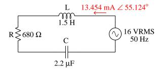
Now we are prepared to calculate voltages across each of the passive components using Ohm's Law, multiplying these polar complex quantities by finding the products of the magnitudes and sums of the angles:
