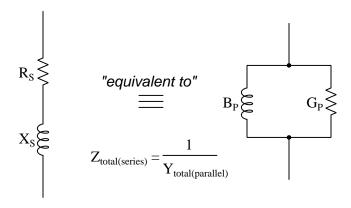
These sums may be computed using scalar numbers, with series impedance (Z) being the Pythagorean sum of R and X being Z, and parallel admittance (Y) being the Pythagorean sum of G and B:
