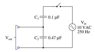
Describe what advantages a capacitive voltage divider might have over a resistive voltage divider.
