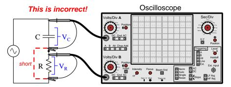
However, the fact that both of the oscilloscope's input channels share a common ground (chassis) connection means that there will be a short-circuit imposed between the two ground clips in this circuit, effectively bypassing the resistor!
