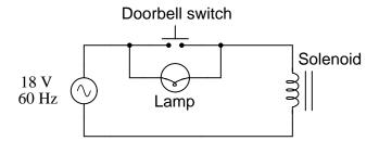
Suppose that such a doorbell circuit suddenly stops working one day, and the home owner assumes the power source has quit since the bell will not ring when the button is pressed and the lamp never lights. Although a dead power source is certainly possible, it is not the only possibility. Identify another possible failure in this circuit which would result in no doorbell action (no sound) and no light at the lamp.
