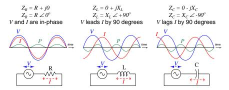
Graphical expressions of complex-number resistance and reactance values are called *phasor diagrams*. Three such diagrams illustrate the difference between a 50  $\Omega$  resistor versus an inductor having 50  $\Omega$  of reactance and a capacitor also having 50  $\Omega$  of reactance:
