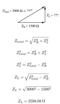
Assuming a pure inductance (i.e. no parasitic resistance or capacitance within its windings), the magnitude of its impedance  $(Z_L)$  will be equal to its reactance  $(X_L)$ . Thus,
