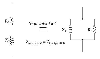
We know that while resistances and reactances add (as phasor quantities) in series, the same cannot be said in parallel. However, the reciprocal of resistance (called *conductance*, G) and the reciprocal of reactance (called *susceptance*, B) do add as phasor quantities in parallel to yield a sum known as *admittance* (Y) which is the reciprocal of impedance (Z):
