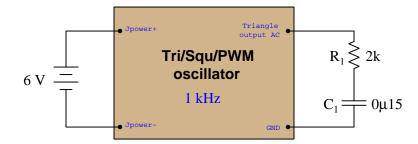
Connected to the RC network, frequency was measured using a Fluke model 87-III multimeter and adjusted to 1 kHz, and then total voltage measured across the series  $R_1 \leftrightarrow C_1$  combination as 233.0 mVAC.
