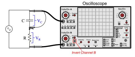
By intentionally inverting Channel B's displayed waveform, we "un-do" the 180° inversion imposed by the necessary probe connection with respect to the oscilloscope's common ground. With this feature engaged, we may correctly interpret the oscilloscope's display to discern the true phase shift between these two components' voltages.
