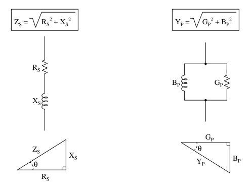
If these two circuits are truly equivalent to one another, having the same total impedance, then their representative triangles should be geometrically similar (identical angles, same proportions of side lengths). With equal proportions,  $\frac{R_S}{Z_S}$  in the series circuit triangle should be the same ratio as  $\frac{G_P}{Y_P}$  in the parallel circuit triangle, that is  $\frac{R_S}{Z_S} = \frac{G_P}{Y_P}$ .
