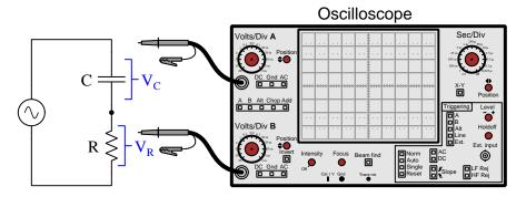
How should we connect the oscilloscope's probes across each of the components to perform this test? At first it may seem like this would be the best way, connecting each probe similarly across the two components:
