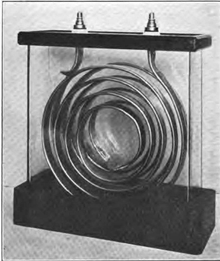
FIGURE 15—Twenty-five Microhenry Inductance Coil Unit, 200 Amperes.
