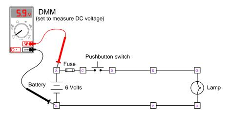
A voltage of 5.9 Volts seems a bit weak, but should still be sufficient to cause a 6-Volt lamp to illuminate. Certainly a much lower measurement (e.g. less than 1 Volt) would be conclusive of a dead battery, but can we be so sure about a 5.9 Volt measurement representing a battery with useful life remaining?
