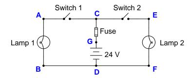
Identify the likelihood of each specified fault for this circuit. Consider each fault one at a time (i.e. no coincidental faults), determining whether or not each fault is compatible with *all* measurements and symptoms in this circuit.
