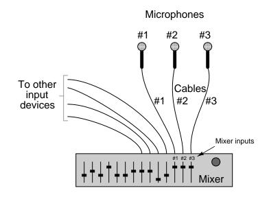
This system has a problem, though. Microphone #2 seems to be "dead," meaning that channel #2 on the mixer does not register any signal when the singer sings into that microphone. All the other channels are working just fine, though.
