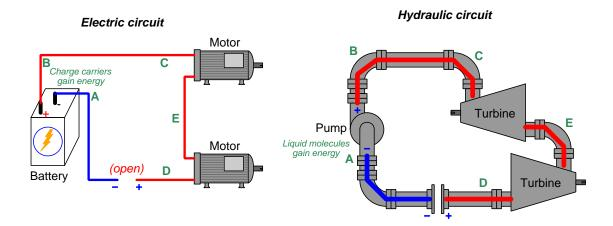
Note how the only portion with low potential lies between the "-" side of the source and the "opened" pathway. All other portions of each circuit immediately equalize in potential to be the same (high). Each load experiences zero difference of potential across it, since the flow ceases everywhere as a result of the "open", but a potential difference does exist across the "open".
