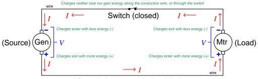
Charges neither lose nor gain energy along the conductive wire
