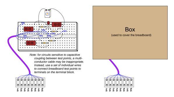
Using the troubleshooting harness means the diagnostician must rely on voltage measurements taken from terminals on the block. This is quite challenging, as not even the shapes of the components may be seen with the box in place. A copy of the circuit's schematic diagram with test points labeled (TP1 through TPn) is the only guide.
