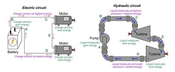
"Potential" may be thought of as *specific potential energy*, or the amount of potential energy possessed by a certain quantity of mobile fluid particles. In the case of electricity, electric potential is the number of Joules of potential energy carried by one Coulomb  $(6.2415 \times 10^{18})$  of charge carriers. In the case of hydraulic systems, fluid potential is better known as *pressure* and is the number of Joules of potential energy carried by one cubic meter of the fluid.
