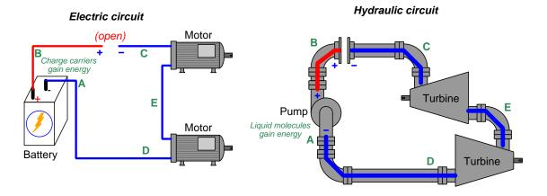
Now we will place an "open" (i.e. a blockage to flow) on the upper portion of each circuit:
