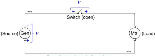
Charges neither lose nor gain energy along the conductive wire
