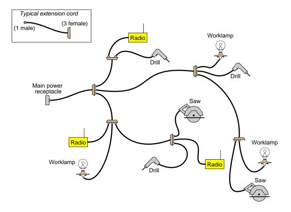
Despite this dangerous wiring, all tools have functioned so far without trouble. Then suddenly both the worklamp and the circular saw in the lower-right corner of the illustration stop working. All the other tools continue to function properly.
