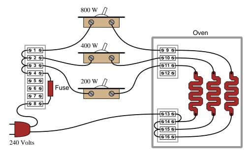
Suppose someone calls you over the telephone to request your diagnostic assistance with this oven. They tell you the 200-Watt switch didn't appear to work: when they turn on that switch by itself, the oven remains at room temperature. Based on this information, the following faults should immediately come to mind as possibilities:
