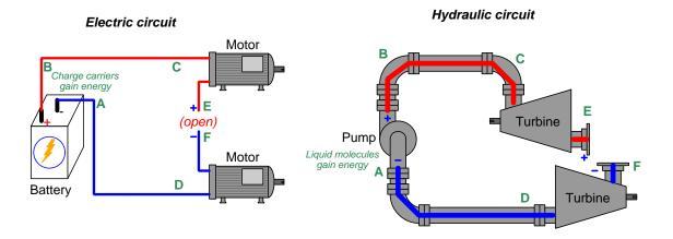
Our last "open" will be placed between the two loads in each circuit:
