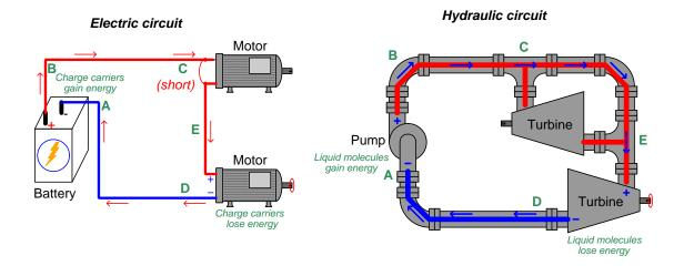
Making both ends of the upper load "common" to each other ensures equipotentiality, robbing the upper loads of any potential difference. This means the flow will not lose any energy going past the shorted load, and instead will deliver all its energy to the lower load which still provides resistance to the flow and is therefore able to extract energy from the flow.
