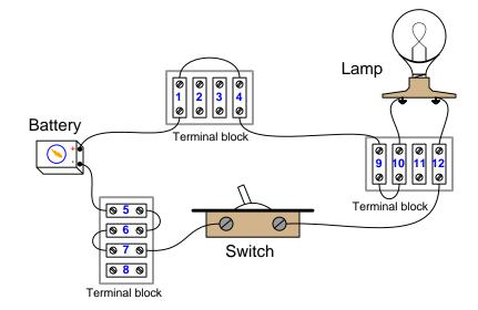
Determine whether or not voltage should be present between the following pairs of terminal block points with the switch in the ON position:
