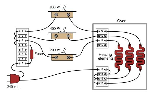
With three differently-sized heating elements (200 watt, 400 watt, and 800 watt), the oven power may be set in seven discrete steps by turning on specific combinations of switches: 200 watts, 400 watts, 600 watts, 800 watts, 1000 watts, 1200 watts, and 1400 watts.
