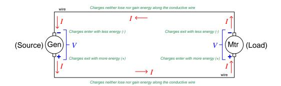
Generators and motors are merely energy-transfer devices: the generator receives mechanical energy from some "prime mover" machine spinning its shaft to impart to electric charges in the circuit, while the motor extracts energy from passing charges to perform useful mechanical work.
