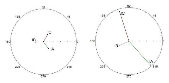
First, identify the phase rotation of this power system based on the color-coding of the phasors. Is it ABC or is it CBA? How are you able to determine this fact.
