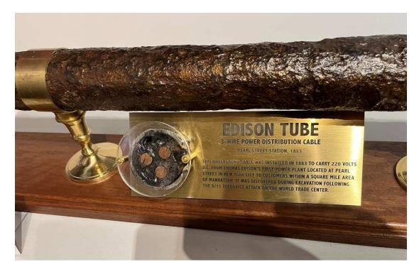
A cross-section of this cable shows the three copper conductors encased in tar within the metallic sheathing of the cable. Despite the obvious corrosion evident on the outside of the cable, it is clear that the copper conductors themselves are well-preserved.
