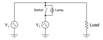
Imagine a condition where generator  $V_1$  is operating and powering the load, but generator  $V_2$  is stopped with its disconnecting switch in the open position. In this condition the lamp will glow steadily, operating on the difference of potential between the power line (full AC voltage) and the idle generator  $V_2$  (0 Volts).
