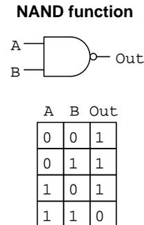
Next we will examine equivalent relay circuits in schematic form fulfilling each of these logic functions, interpreting a “1” state as *energized* and a “0” state as *de-energized*. Normally-open pushbutton switches will provide input signals to our logic function, while a lamp provides visual output signal confirmation.
