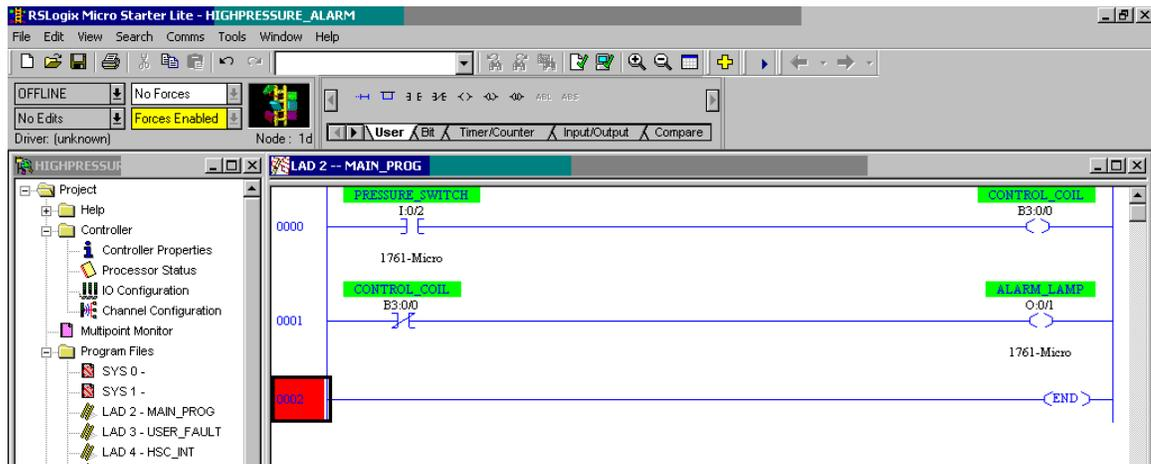
Suppose a fluid pressure of 36 PSI is applied to the pressure switch. This is less than the switch's trip setting of 50 PSI, leaving the switch in its "normal" (closed) state. This sends power to input I:0/2 of the PLC. The contact labeled I:0/2 drawn in the ladder-logic program of the PLC acts like a relay contact driven by a coil energized by input terminal I:0/2. Thus, the closed pressure switch
