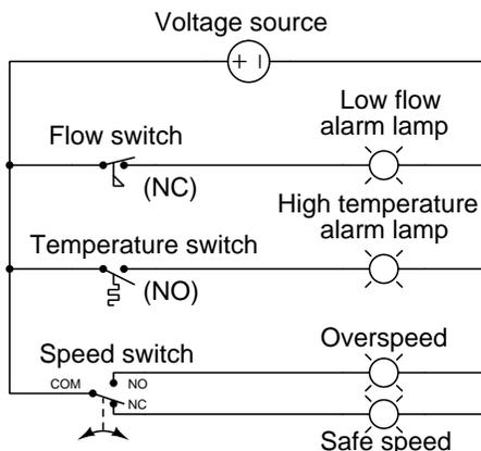
Note the COM, NO, and NC labeling of this switch’s three terminals, denoting “Common”, “Normally-Open”, and “Normally-Closed”, respectively. As with the other two switches, these contact labels as well as the switch symbol itself as drawn in the diagram represent the switch’s state *when at rest*. This is strict convention in electrical switching circuits: the “normal” state of any switch is defined by a condition of minimal stimulus, and this is always how it is drawn.
