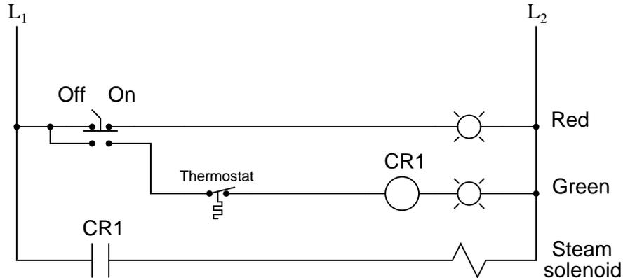
This mistake is very common among students new to relay ladder-logic diagrams. Explain what the mistake is, and draw a corrected version of this relay circuit.
