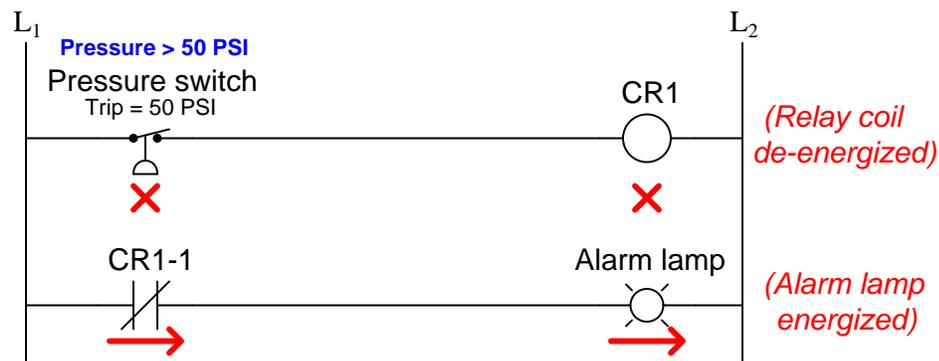
Now that there is sufficient fluid pressure applied to the switch to actuate it, its contact is forced into the actuated state which for this "normally-closed" switch is open. This open condition de-energizes relay coil CR1, allowing relay contact CR1-1 to spring-return to its normal status (closed), thus sending power to the alarm lamp. From this analysis we see that the lamp fulfills the function of a *high pressure alarm*, energizing when the applied pressure exceeds the trip point.
