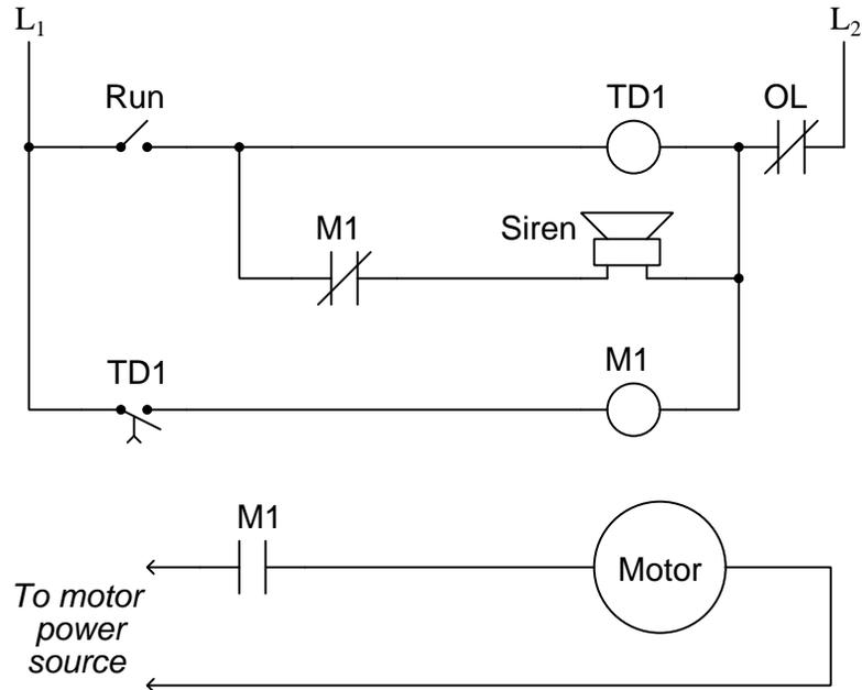
Study this ladder logic diagram, then explain how the system works.
