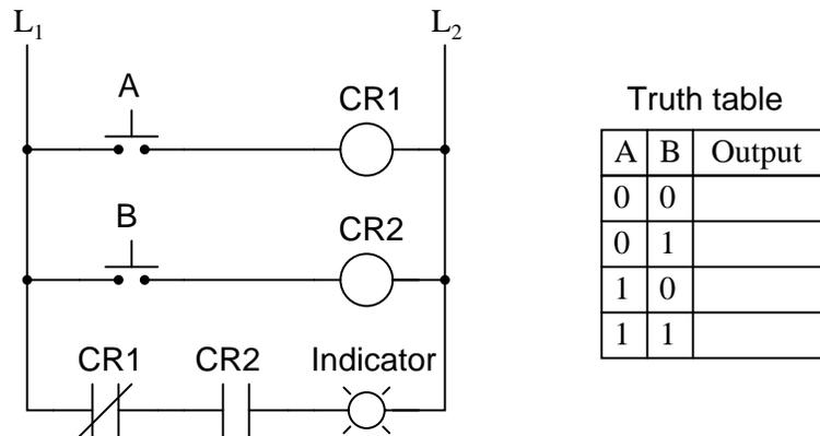
Also, demonstrate how to apply the annotation techniques described in the Tutorial to this circuit as you determine what its output will be for each input condition.
