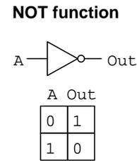
By combining OR and AND functions with inversion (the NOT function), we may form two more common “building-block” logical functions, *NOR* and *NAND*:
