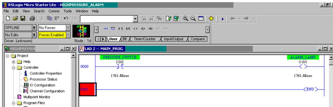
The effect is the same: the PLC output O:0/1 will activate whenever input I:0/2 de-energizes (whenever the pressure switch is opened by a high pressure), turning on the alarm lamp in a high-pressure condition. In a low-pressure condition, the energized input I:0/2 forces the virtual normally-closed contact I:0/2 to open, thus de-energizing the PLC’s output O:0/1 and turning the alarm lamp off.
