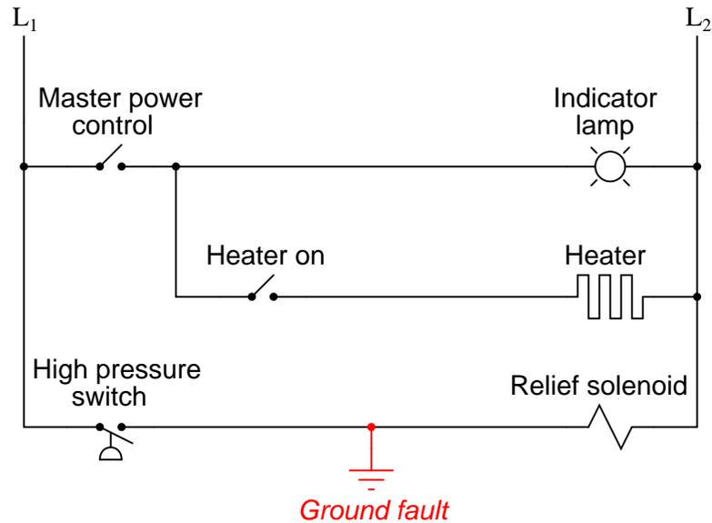
What would be the result of this ground fault? Would it matter if the L1/L2 power connections were reversed?
