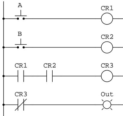
It is very important to realize that the diagonal line drawn through a relay contact represents its *normal state* and not necessarily its *present state* or *typical state*. In fact, this is one of the most common misconceptions for students first encountering ladder diagrams.
