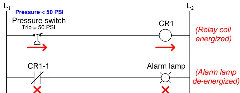
Using arrow and "X" symbols again to represent the presence or absence of power in this circuit, we will now analyze its status with an applied switch pressure greater than 50 PSI:
