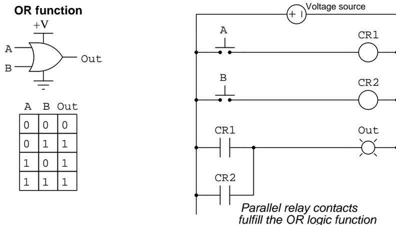
This ladder-style diagram is so much clearer than the schematic-style diagram previously shown, owing to the complete absence of any crossing lines. The parallel connection between the two relays' normally-open contacts is quite obvious in the ladder diagram, and the lack of dashed lines connecting relay contacts to their respective coils unclutters the illustration.
