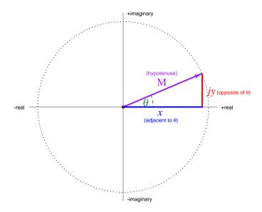
The polar angle  $\theta$  may be calculated three different ways, based on side y of the triangle being opposite of  $\theta$  and side  $\theta$  and adjacent to angle  $\theta$ , knowing that the tangent function is the ratio between opposite and adjacent and hypotenuse, and that the sine function is the ratio between opposite and hypotenuse:
