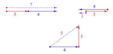
Also explain the significance of these sums: that we may obtain three *different* values of total voltage (7 Volts, 1 volt, or 5 Volts) from the same series-connected AC voltages. What does this mean for us as we prepare to analyze AC circuits using the rules we learned for DC circuits?
