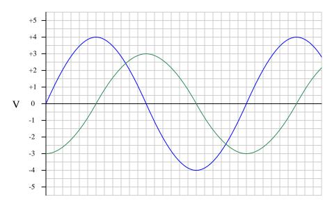
As accurately as possible, determine the amount of phase shift between the two waves, based on the divisions shown on the graph.
