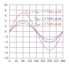
Here we clearly see a sine wave with a peak value of 3  $(V_{AB})$  along with a sine wave with a peak value of 4  $(V_{BC})$ , added together to make a third sine wave having a peak value of 7. This is rather intuitive: if we imagine these two sine waves adding together at every point in time, the sum must be zero at that exact angle when both waves cross zero, and the sum should peak at 7 Volts when each source is at its respective peak. Algebraic factoring proves this as well:
