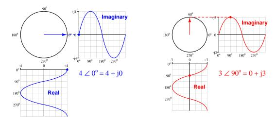
The sum of 4 + j0 and 0 + j3 is simply 4 + j3. As it so happens, a phasor with polar magnitude of 5 and an angle of  $36.87^{\circ}$  will have these equivalent real and imaginary values:
