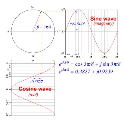
The sine wave exists as the vertical projection of the rotating phasor on the "imaginary" (j or i) axis, while the cosine wave exists as the horizontal projection of that same phasor on the "real" axis. At the particular angle arbitrarily chosen for this example ( $3\pi/8$  radians) the vertical quantity happens to be j0.9239 while the horizontal quantity happens to be 0.3827.
