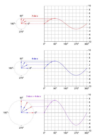
This graphically represents our first AC scenario, where a 3 Volt sine wave and a 4 Volt sine wave at the same frequency and in-phase with each other add together to make a 7 Volt sine wave.
