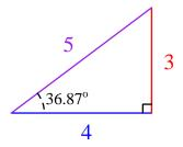
This is how two phase-shifted quantities add together: represented as line-segments having length (magnitude) and direction (angle), the resultant (sum) is another line-segment joining the starting-point to the end-point.
