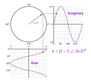
While it may be simple to plot horizontal and vertical phasors such as  $4 \angle 0^o$  and  $3 \angle 90^o$  onto graphs, it is far from obvious how to plot just the right phasor to give us a result having both non-zero real and imaginary values. Symbolic conversion from rectangular form into polar form requires some right-triangle trigonometry, as shown below:
