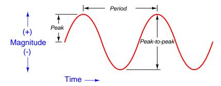
An AC voltage, for example, would possess a certain peak, peak-to-peak, and/or RMS voltage value as well as a period (measured in seconds) and a frequency (measured in cycles per second or Hertz). A greater magnitude appears "taller" on the vertical axis of a graph and a greater frequency appears "compressed" on the horizontal axis of a graph (i.e. more cycles within the same amount of time, or a shorter period).
