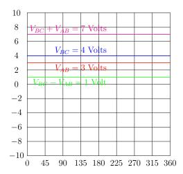
The sum of the 4 Volt line and the 3 Volt line is a 7 Volt line; the difference between the 4 Volt line and the 3 Volt line is a 1 Volt line.
