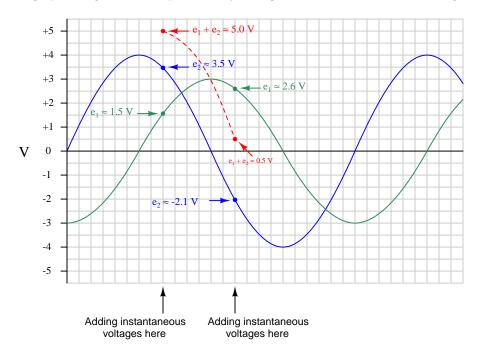
Calculate the peak value of the resultant (sum) sine-wave, and compare this with the peak values of the two original sine waves.
