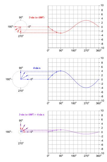
Note how the phasors of the 3 Volt sine wave begin at 180 degrees and end at 270 degrees because that function is offset 180 degrees from the 4 Volt sine wave. The sum of these two sine waves, of course, is a sine wave having a peak value of only 1, since for every value of x the two phasors are pointing in opposite directions of each other and therefore subtract.
