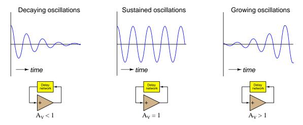
Sketch locations of poles for each of these oscillator loop-gain conditions, qualitatively placing "X" marker(s) for those locations on the s plane:
