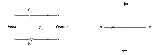
$$\label{eq:Transfer} \text{Transfer function} = \frac{C_1}{sRC_1C_2 + C_1 + C_2}$$
