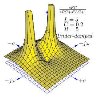
We clearly see two poles once again, but neither of them are located on an axis. These represent two complex values for s describing the circuit's behavior with zero input. The non-zero imaginary  $(j\omega)$  part of s tells us the circuit has the ability to self-oscillate. The negative, real  $(\sigma)$  part of s tells us these oscillations decrease in magnitude over time. Using the quadratic formula to solve for these two poles:
