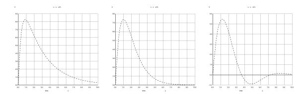
Note how the under-damped case (right) is the only one where the output signal actually oscillates about the 0-Volt axis. In the critically damped case (middle) the output decays rapidly to zero, while in the over-damped case (left) the output's decay to zero is more gradual.
