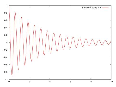
This shows a higher-frequency and faster-decaying waveform than any of the others. Shown as a point on the s plane:
