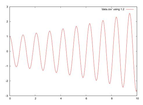
This shows a waveform with a growing amplitude over time, since  $\sigma$  (the growth/decay rate) is a positive number. Shown as a point on the s plane:
