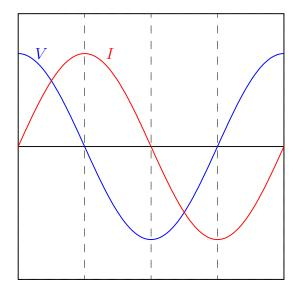
Therefore, when we apply a sinusoidal current through a pure inductor, the voltage waveform is also a sinusoid but phase-shifted by 90 degrees leading. In other words, *voltage leads current by 90 degrees for a pure inductance*.
