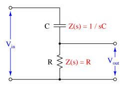
$$\text{Transfer function} = \frac{V_{out}(s)}{V_{in}(s)} = \frac{R}{R + \frac{1}{sC}} = \frac{R}{R + \frac{1}{(\sigma + j\omega)C}}$$
