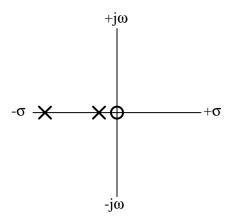
If L=100 mH and  $C=68~\mu\mathrm{F}$  and  $R=27~\Omega$ , then we have an under-damped condition:
