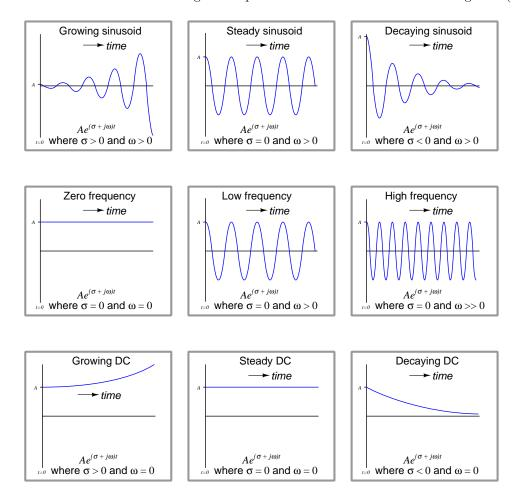
Simple frequency, whether f or  $\omega$ , merely describes the rate at which an AC signal oscillates. Complex frequency, by contrast, is additionally able to describe growth, decay, or stability. As such it is a more general and indeed more useful way to describe signals.
