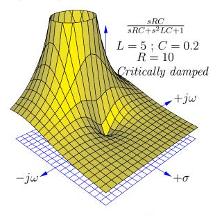
As expected, a single zero appears at s=0, and a single pole at s=-1+j0. Thus, this circuit has a decay rate of -1 time constants per second ( $\tau=1$  second) as seen when we use the quadratic formula to solve for s:
