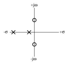
If L = 100 mH and  $C = 68 \mu F$  and  $R = 27 \Omega$ , then we have an under-damped condition:
