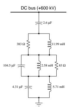
Identify the type of filter this is (e.g. low-pass, high-pass, band-pass, or band-stop) and also which harmonics of 60 Hz it is designed to attenuate.
