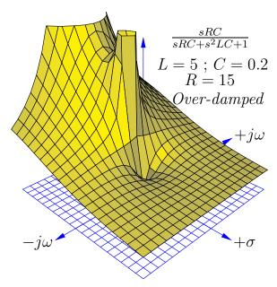
We clearly see two poles<sup>13</sup> centered along the  $\sigma$  axis in this plot, representing the two real roots of the transfer function's denominator. Again, we will use the quadratic formula to solve for these two values of s:
