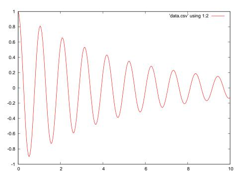
This shows a waveform with a more rapidly decaying amplitude over time, since  $\sigma$  (the growth/decay rate) is a stronger negative number. Shown as a point on the s plane:
