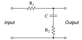
This network's transfer function may be written using the voltage divider equation, placing the series impedance of C and  $R_2$  over the total network impedance as seen from the input terminals. First, writing an s-domain impedance equation for C and  $R_2$ :
