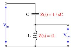
Writing the transfer function for this tank circuit is (once again) a matter of expressing the ratio between the output component's impedance versus the total circuit impedance:
