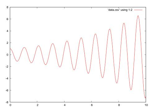
This shows a waveform with a more rapidly growing amplitude over time, since  $\sigma$  (the growth/decay rate) is a stronger positive number. Shown as a point on the s plane:
