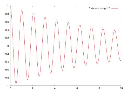
This shows a waveform with decaying amplitude over time, since  $\sigma$  (the growth/decay rate) is negative. Shown as a point on the s plane:
