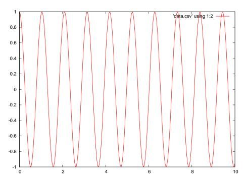
This shows a waveform with constant peak amplitude over time, since  $\sigma$  (the growth/decay rate) is equal to zero. Shown as a point on the s plane:
