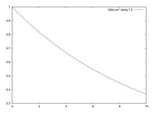
This shows a non-oscillating decay, since  $\sigma$  (the growth/decay rate) is a negative number and  $\omega$  (the oscillation rate) is zero. Shown as a point on the s plane:
