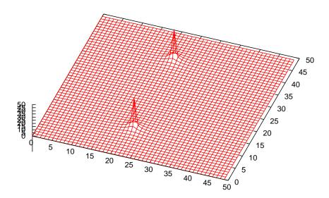
This particular simulation uses increments of 0.04 per second (incr in the C++ code), which is the value of each division (space between lines) on the two horizontal axes. The two poles of this filter network are clearly evident in the three-dimensional plot, but the height of these peaks is quite irrelevant to our purposes. We just want to know how many poles there are, and where those poles are located on the s plane.
