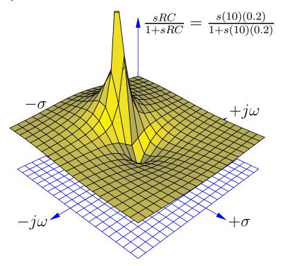
Here we see both the pole at s=-0.5+j0 and the zero at s=0+j0 quite clearly: the pole is a singular point of infinite height while the zero is a singular point of zero height. The three-dimensional surface of the transfer function looks like a rubber sheet that has been stretched to an infinite height at the pole and stretched to ground level at the zero.
