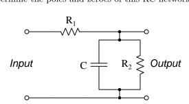
This network's transfer function may be written using the voltage divider equation, placing the parallel impedance of C and  $R_2$  over the total network impedance as seen from the input terminals. First, writing an s-domain impedance equation for C and  $R_2$ :
