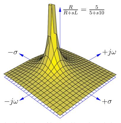
This surface plot makes the meaning of the term "pole" quite obvious: the shape of the function looks just like a rubber mat stretched up at one point by a vertical pole. Here, the "pole" rises to an infinite<sup>5</sup> height at a value of s where  $\sigma = -0.5$  time constants per second and  $\omega = 0$  radians per second. The surface is seen to decrease in height at all edges of the plot, as  $\sigma$  and  $\omega$  increase in value.
