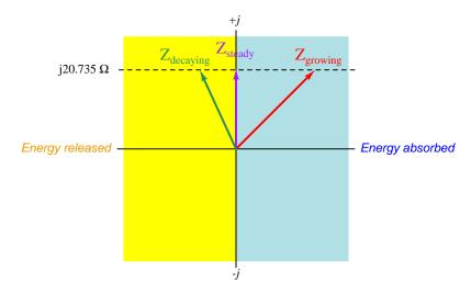
In all three cases the imaginary portion of the impedance is the same (j20.735 Ohms), but the growth or decay of the signal over time contributes a net absorption or net release, respectively, of energy by the inductor over multiple cycles.
