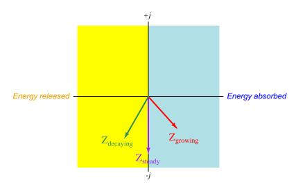
Once again we see how an AC signal of constant magnitude over time results in an impedance phase angle precisely one-quarter cycle, which means the component absorbs and releases energy in equal measure with each cycle. However, when the AC signal's oscillations grow in strength over time the reactive component absorbs more energy than it releases over multiple cycles; when the oscillations decay the component releases more energy than it absorbs over multiple cycles.
