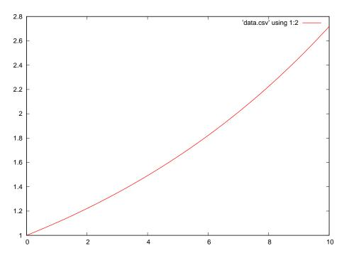
This shows a non-oscillating growth, since  $\sigma$  (the growth/decay rate) is a positive number and  $\omega$  (the oscillation rate) is zero. Shown as a point on the s plane:
