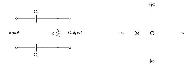
$$\label{eq:Transfer} \text{Transfer function} = \frac{sRC_1C_2}{sRC_1C_2 + C_1 + C_2}$$
