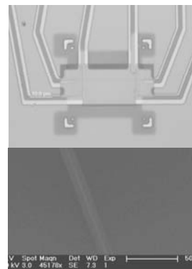
Device micrograph, with ~50nm Si nanowire active region (bottom)
