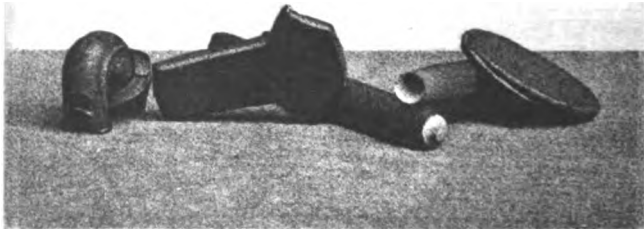
HAMMER AND TENSILE TEST PIECES \frac{3}{4} " RIVETS.
