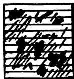
FIRE FELT-HAIR ASBESTOS OR SIMILAR INSULATING MAT'L
