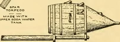
— IRON SPAR — RAM TORPEDO USED ON THE "CHARLESTON"
