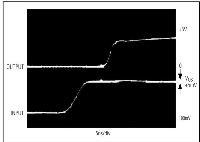
Figure 3.  $t_{pd+}$  Response Time to 5mV Overdrive
