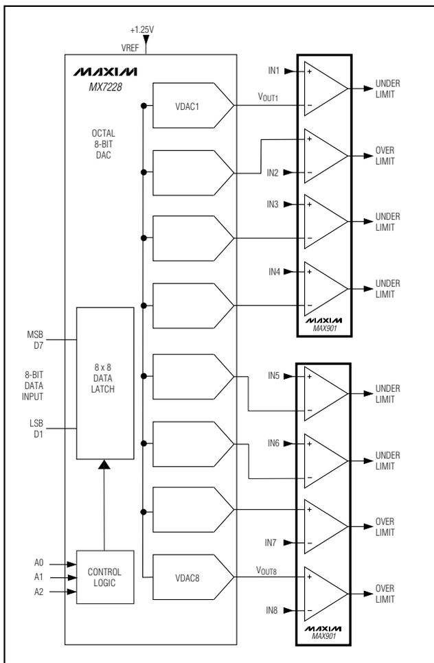
Figure 8. Alarm Circuit Level Monitors Eight Separate Inputs
