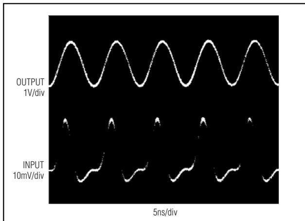
Figure 7. Response to 100MHz Sine Wave Photo
