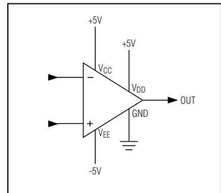
Figure 1C. Split  $\pm 5V$  Supply, Separate Ground
