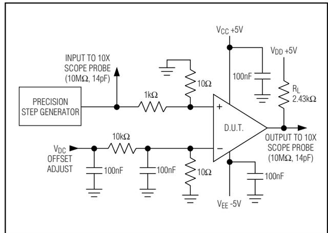
Figure 5. Response-Time Setup
