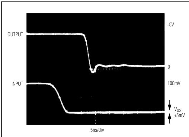
Figure 4.  $t_{pd-}$  Response Time to 5mV Overdrive
