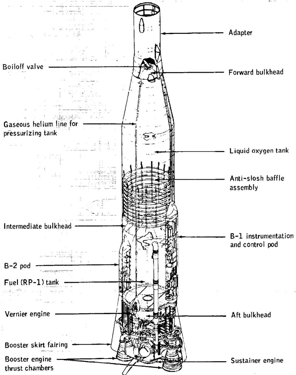
Figure 3.5-1. - Cutaway drawing of target launch vehicle.
