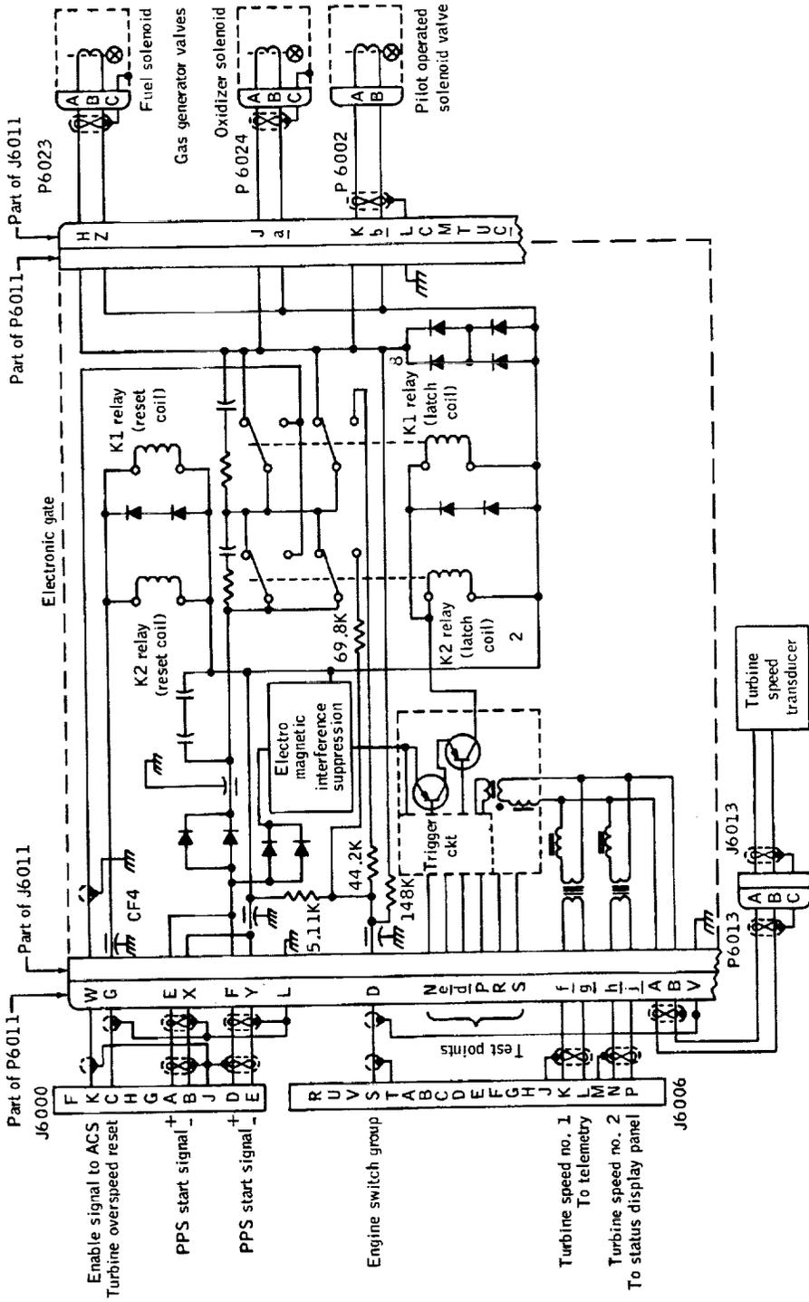
Figure 5. 4. 6-1. - Schematic diagram of the GATV 8247 engine electrical system.
