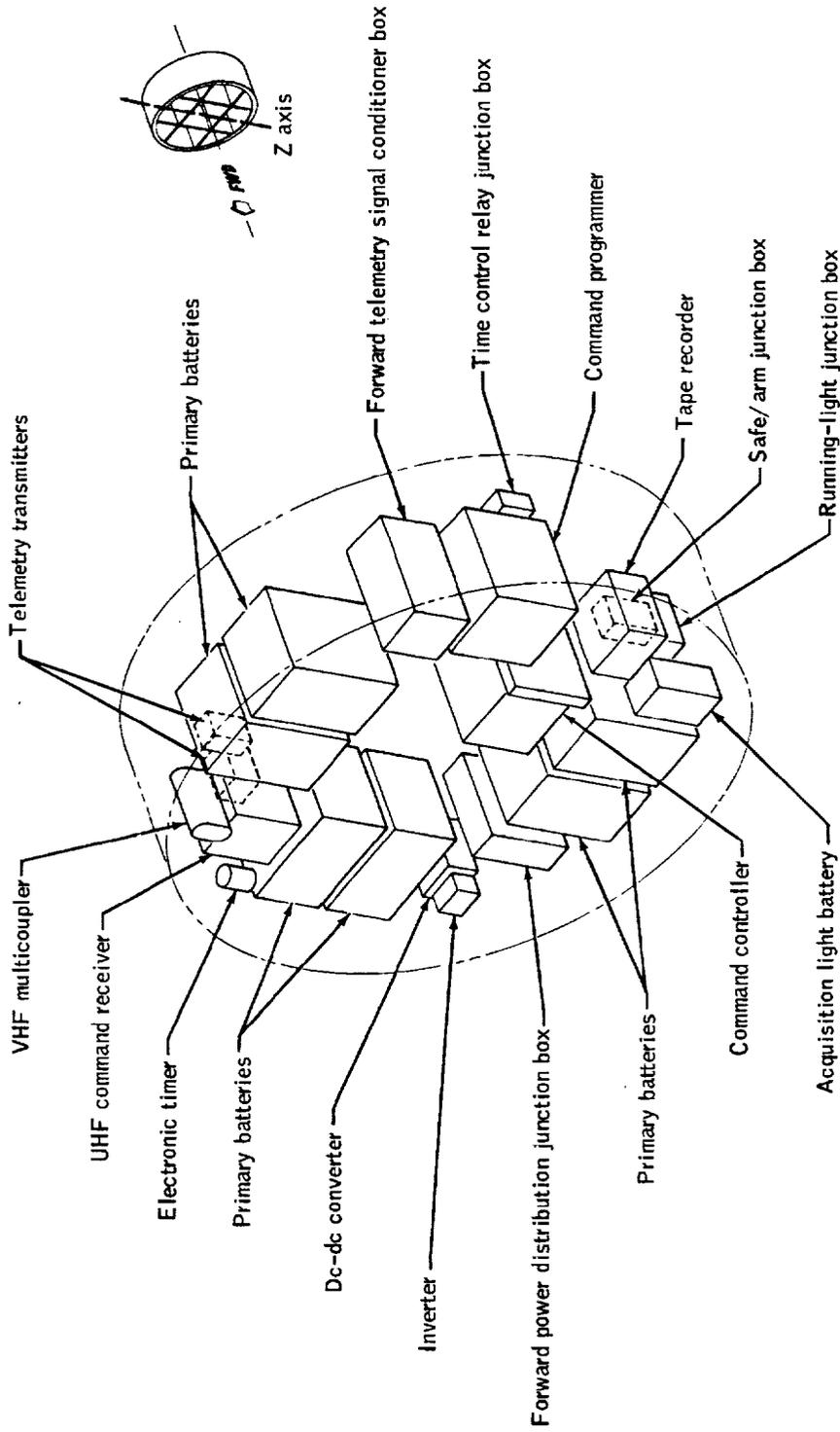
Figure 3.4-3. - Auxiliary forward rack equipment.
