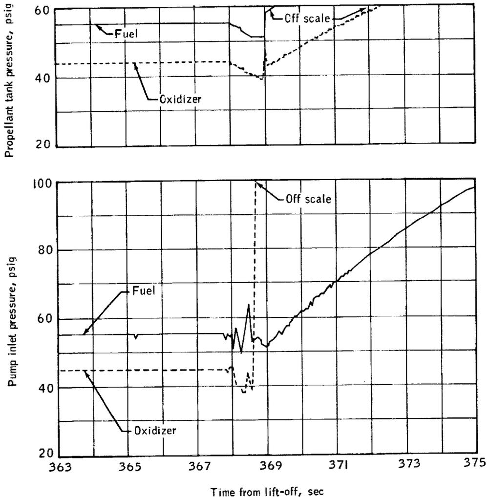
Figure 5.4.2-3. - PPS propellant tank and pump inlet pressure increase.
