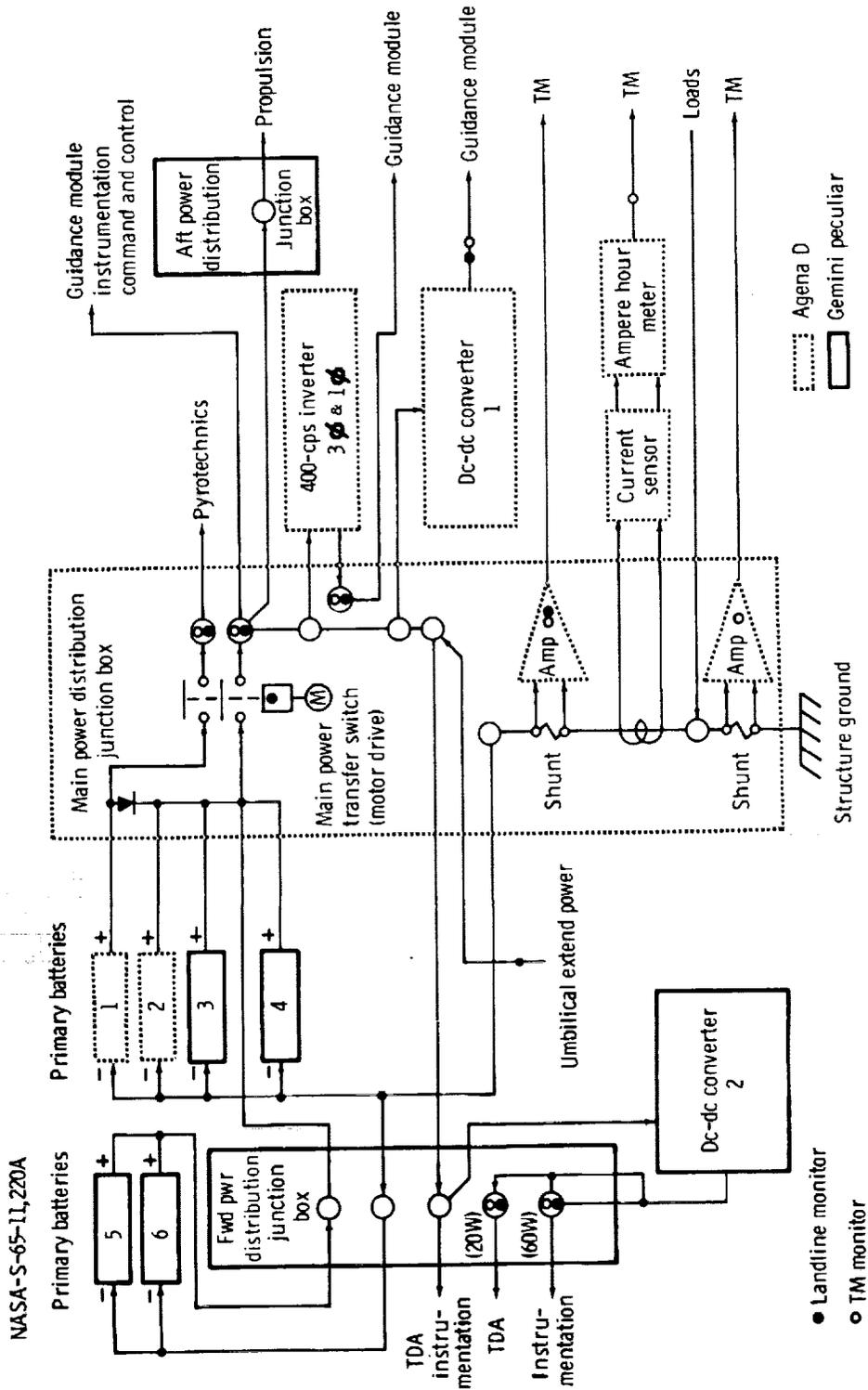
Figure 3.4-12 - GATV electrical system block diagram.
