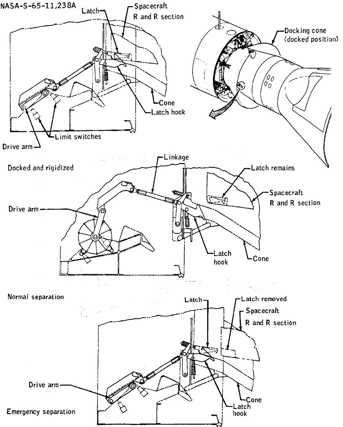
Figure 3.4-8. - Spacecraft - TDA separation sequence .
