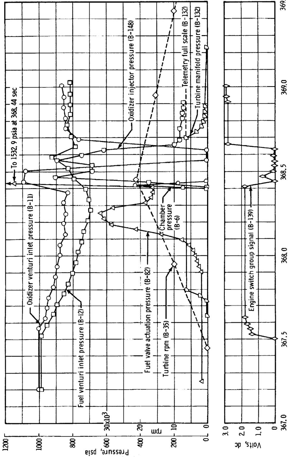
Figure 5.4.2-2. - Primary propulsion system start sequence.
