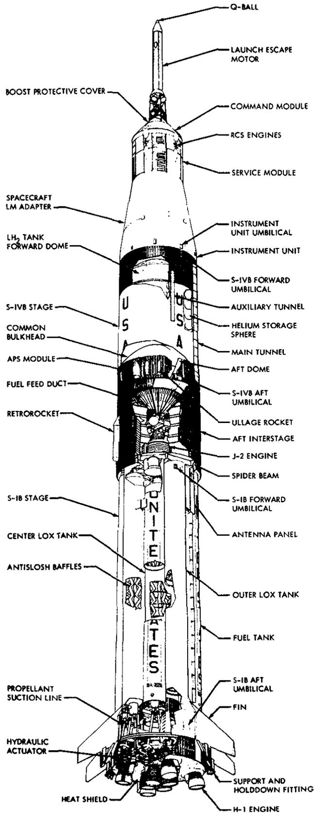
FIRST STAGE -- The Saturn IB booster (S-IB) is 80.2 feet long and 21.5 feet in diameter. Dry weight of the redesigned booster is 84,401 pounds, about 10 tons lighter than the Saturn I booster (S-I).
