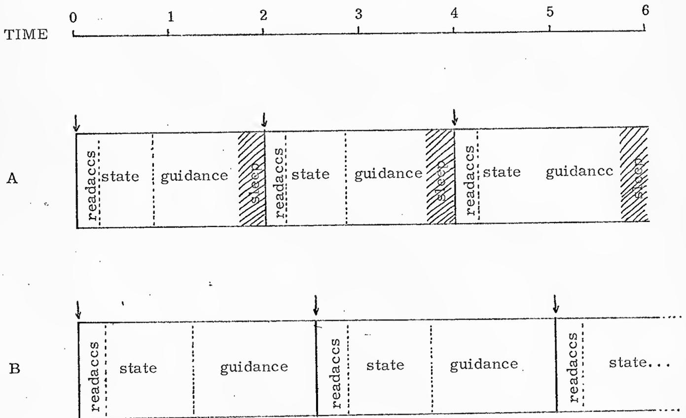
On the next pages are duty cycle and guidance period plots for Landings run on ZERLINA with zero and with 20% TLOSS. After that comes a flowchart of the Servicer job and its auxiliaries.
