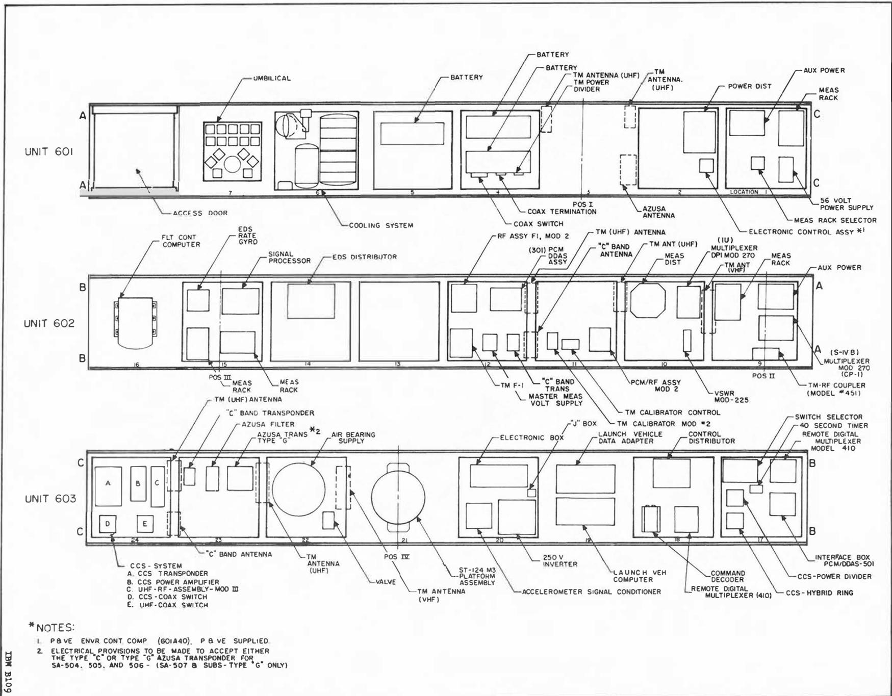
Figure 12.1-5 Saturn V Instrument Unit Equipment Layout, Operational
