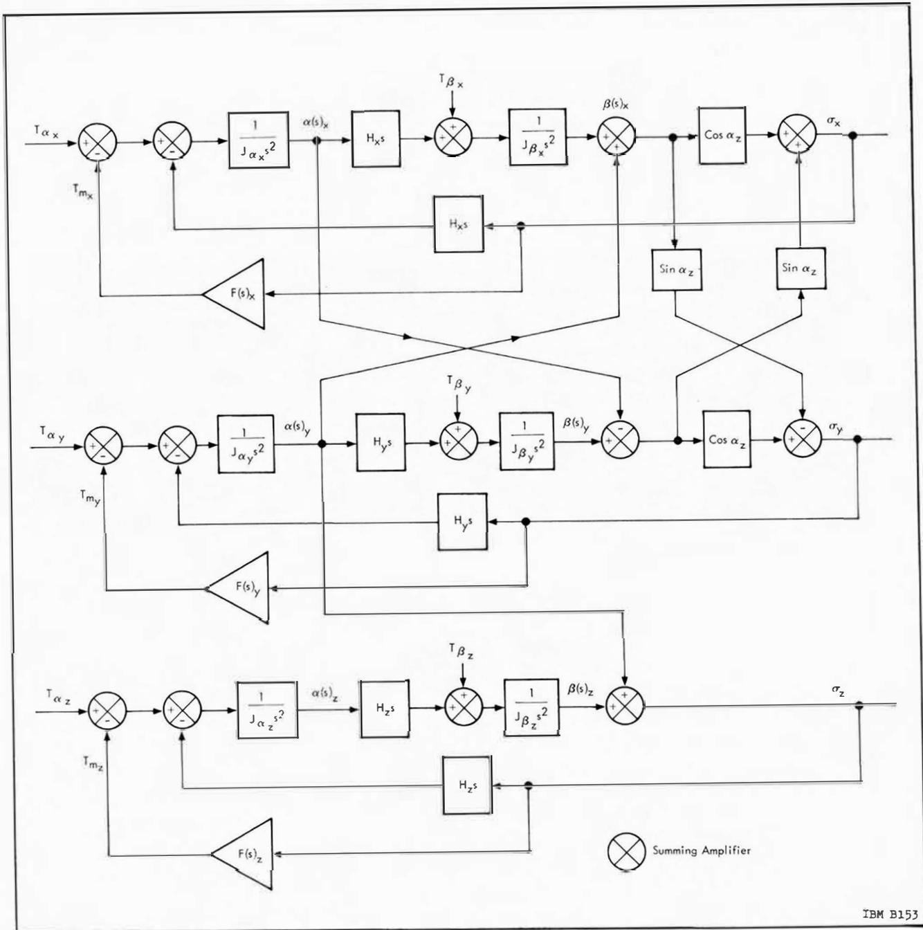
Figure 14. 3-7 Three-axis Inertial Platform Assembly Block Diagram
