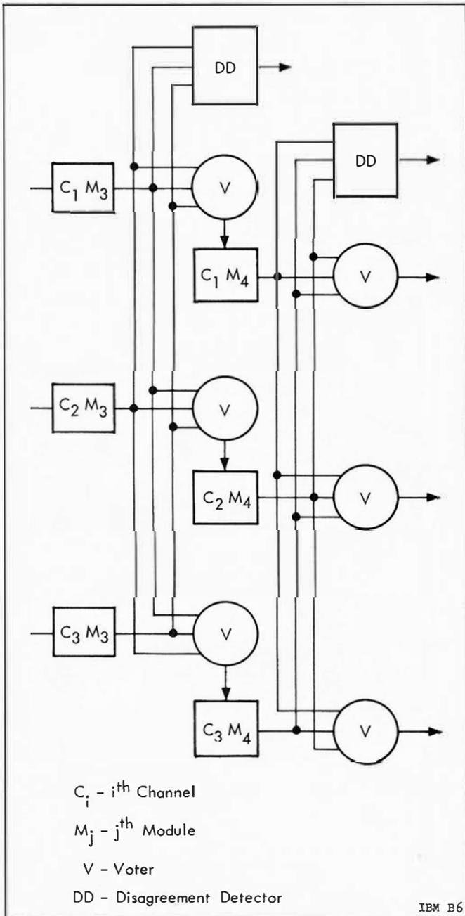
Figure 15.3-2 Triple Modular Redundancy ( TMR )
