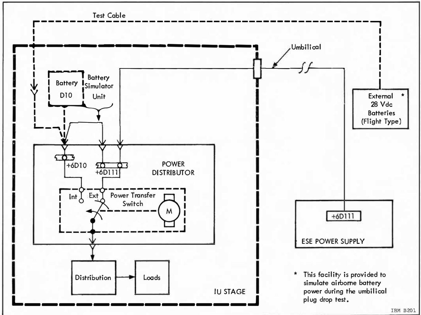
Figure 8.2-4 Ground Checkout Configuration of IU Power Derivation
