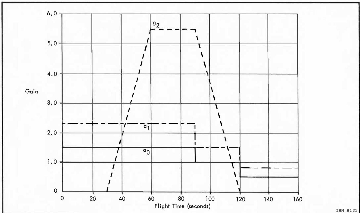
Figure 3.4-4 Typical Gain Program for  $a_0$ ,  $a_1$ ,  $g_2$  Coefficients
