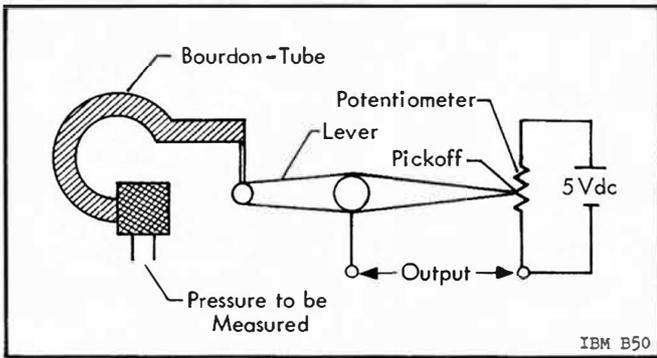
Figure 5. 2-4 Bourdon-tube Potentiometer Type Pressure Transducer
