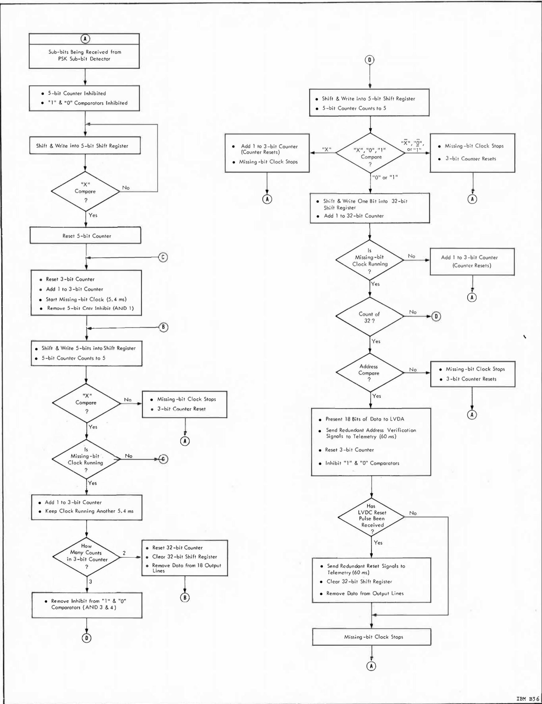
Figure 6.2-13 IU Command Decoder Flow Diagram
