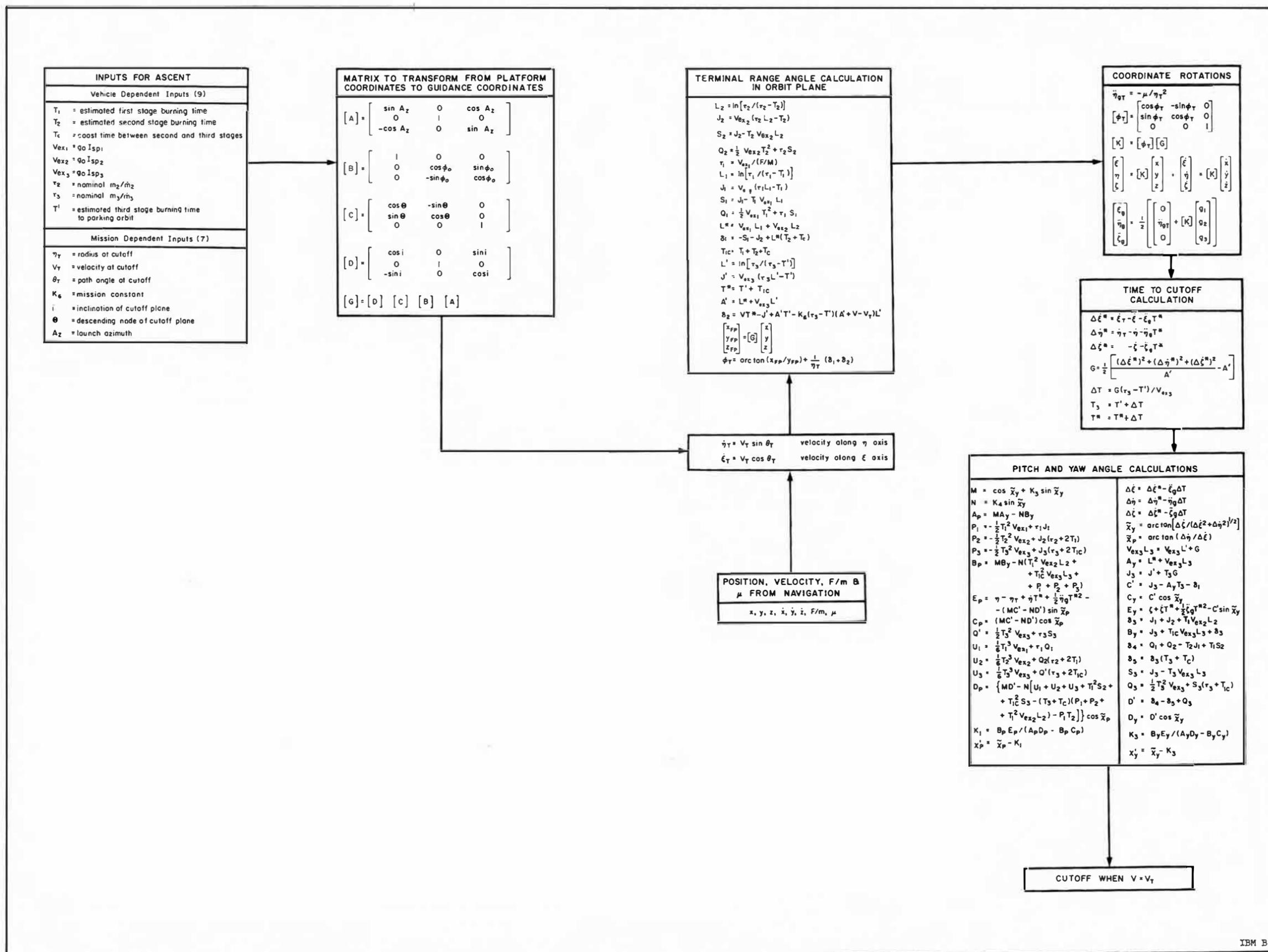
Figure 2.3-2 Iterative Guidance Mode Equations, Flight to Orbit
