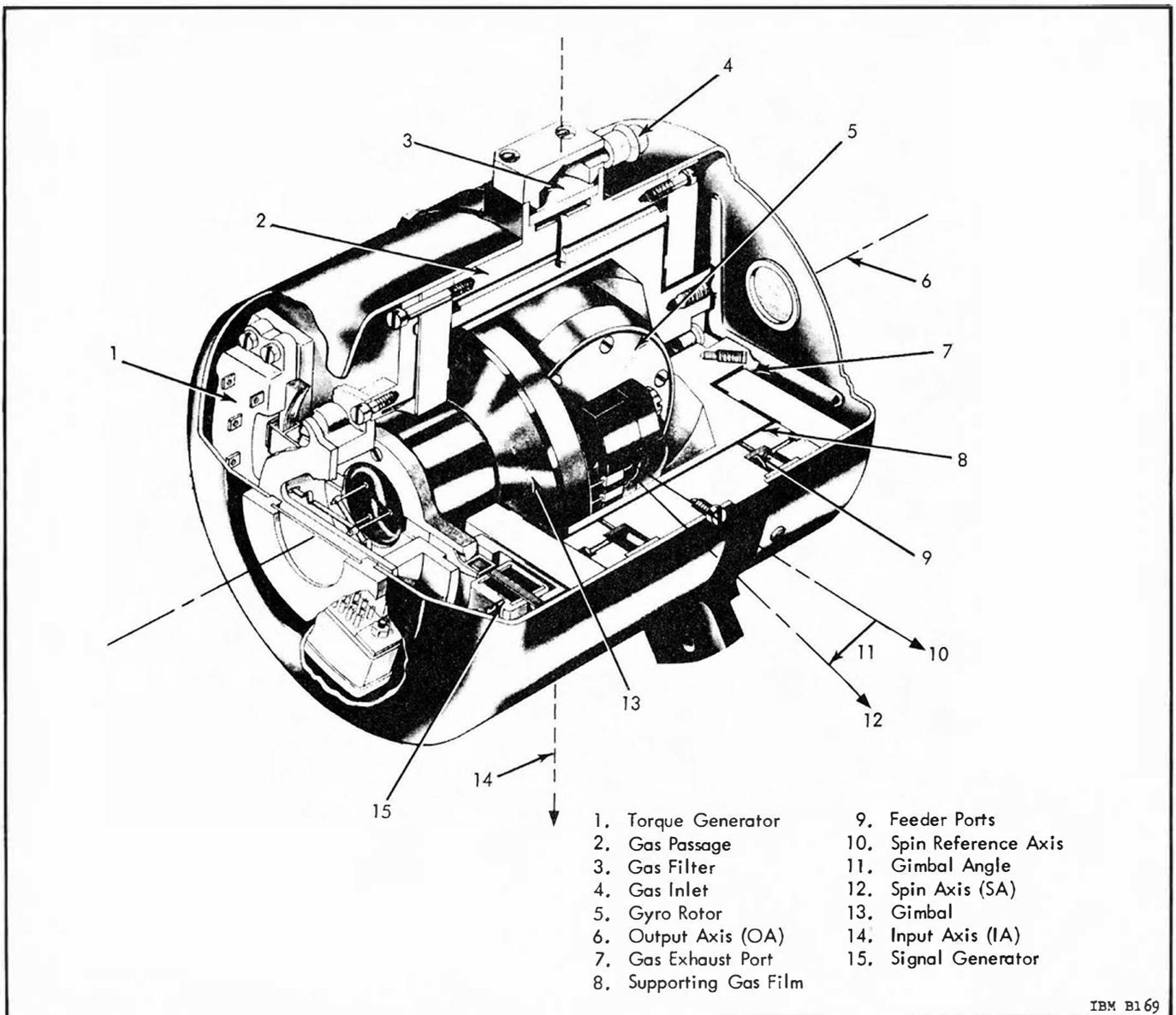
Figure 14. 8-1 Cutaway View of a Single-axis Integrating Gyro
