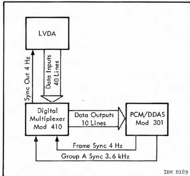
Figure 5. 5-5 Inputs and Outputs of Mod 410 Multiplexer
