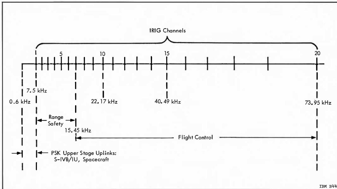
Figure 6.5-2 AN/FRW-2A Modulation Bandwidth Usage
