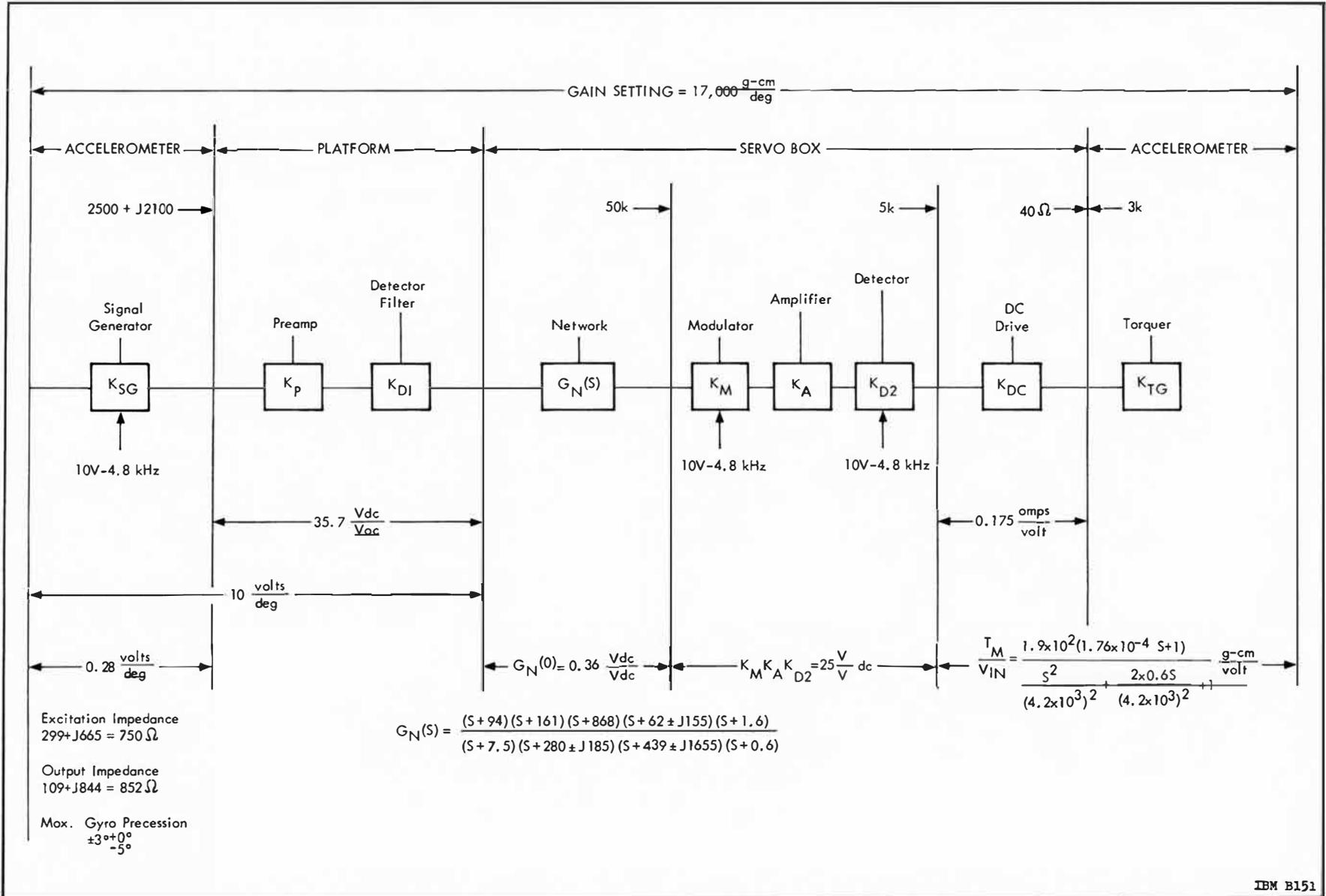
Figure 14.3-5 Accelerometer Electronics Block Diagram
