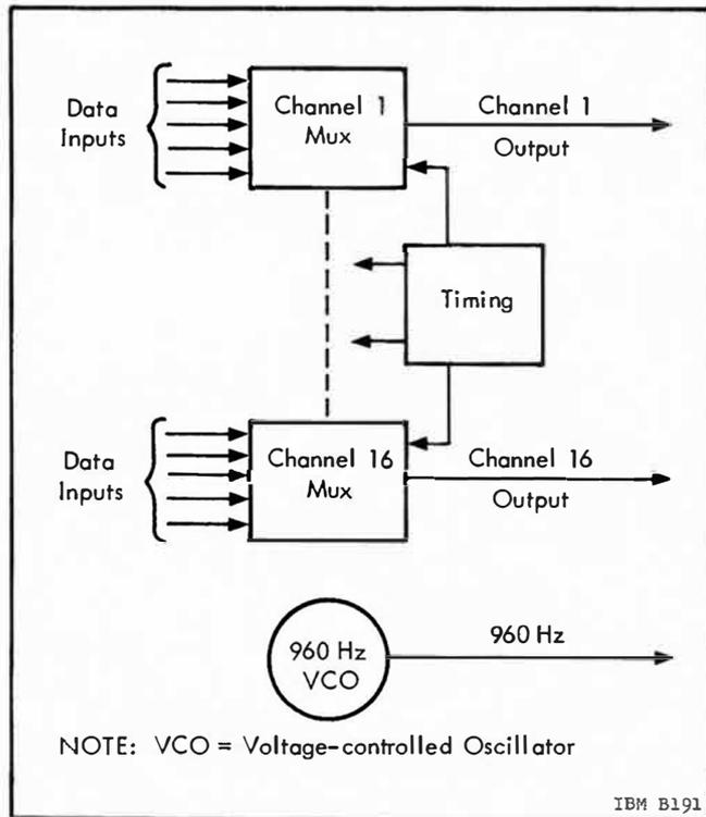
Figure 5. 5-7 Block Diagram of Mod 245 Multiplexer
