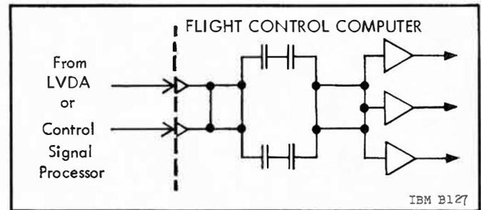
Figure 3.4-9 Redundant Cabling in the Flight Control Computer
