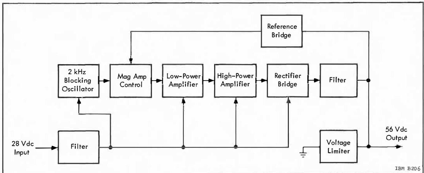
Figure 8.4-1 56 Volt Power Supply Block Diagram
