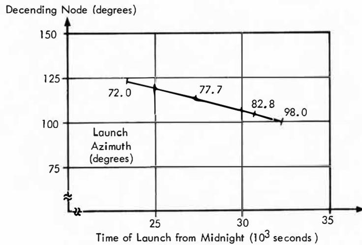
Time of Launch Versus Launch Azimuth for a Typical Launch Window
