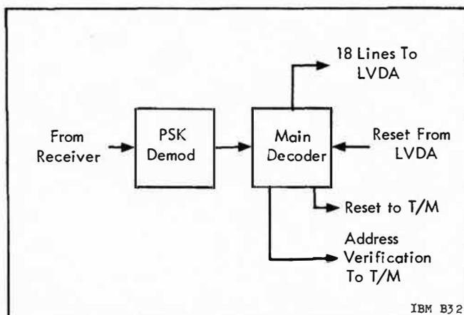
Figure 6.2-9 IU Command Decoder Functional Block Diagram
