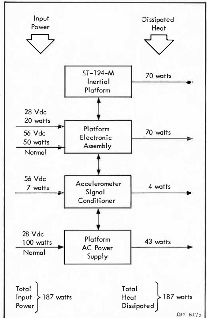
Figure 14.10-1 System Power Requirements and Heat Dissipation
