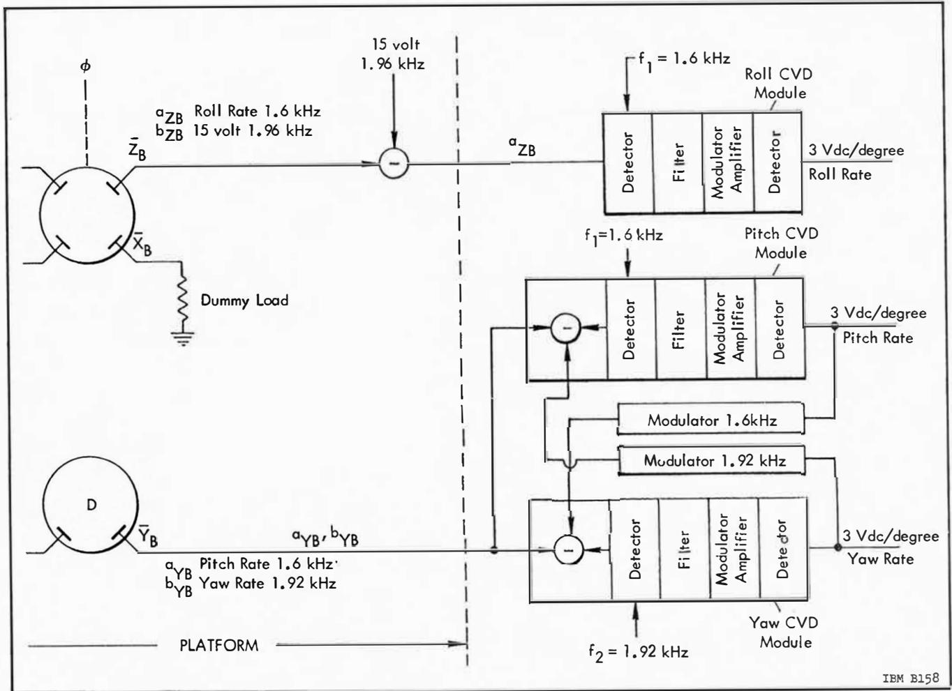
Figure 14. 4-5 Resolver Chain Signal Detection Scheme
