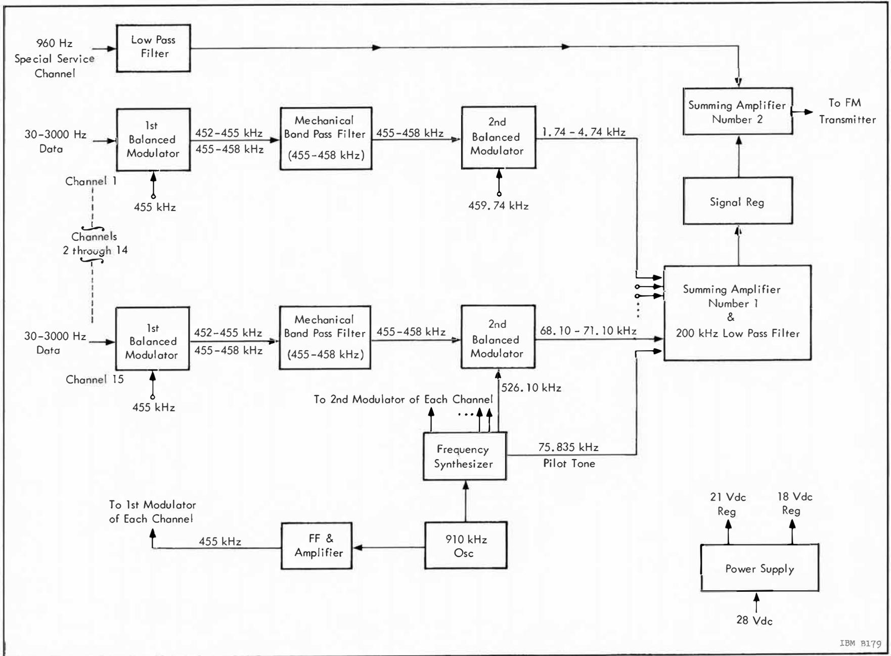
Figure 5. 4-4 Block Diagram of Airborne SS Telemetry Assembly
