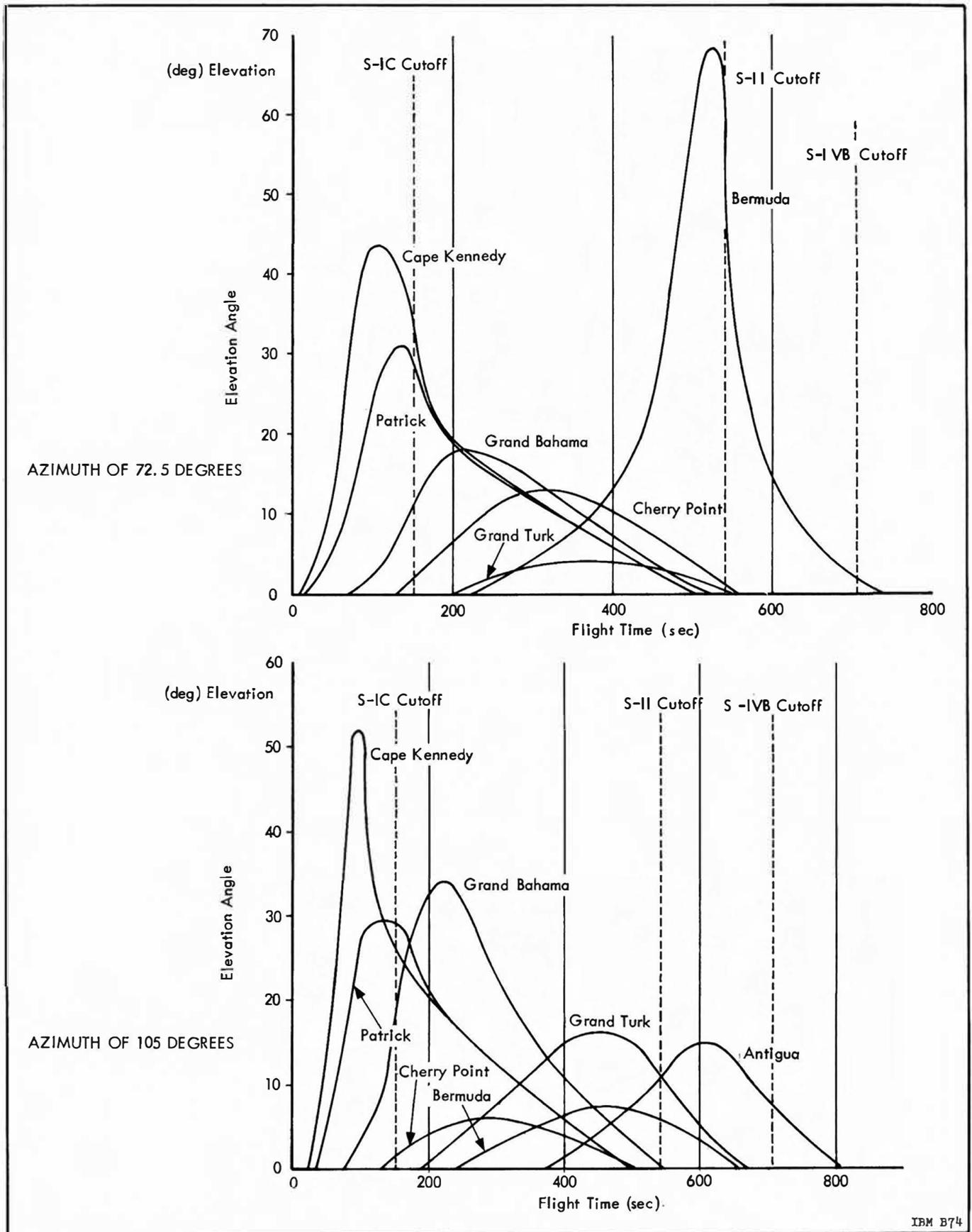
Figure 7.1-2 Station Visibility for Saturn V Powered Flight
