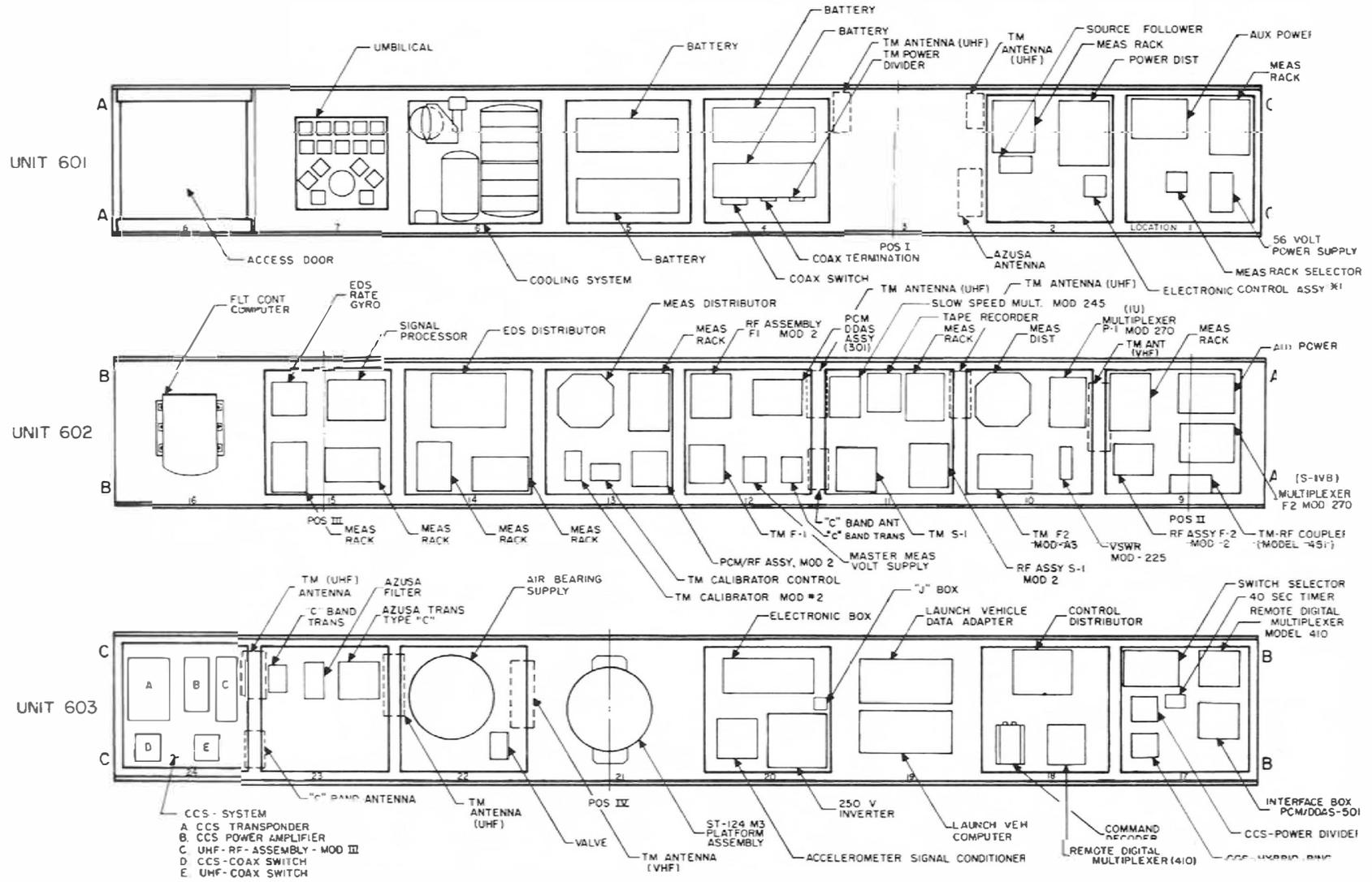
Figure 12.1-3 Saturn V Instrument Unit Equipment Layout, R & D
