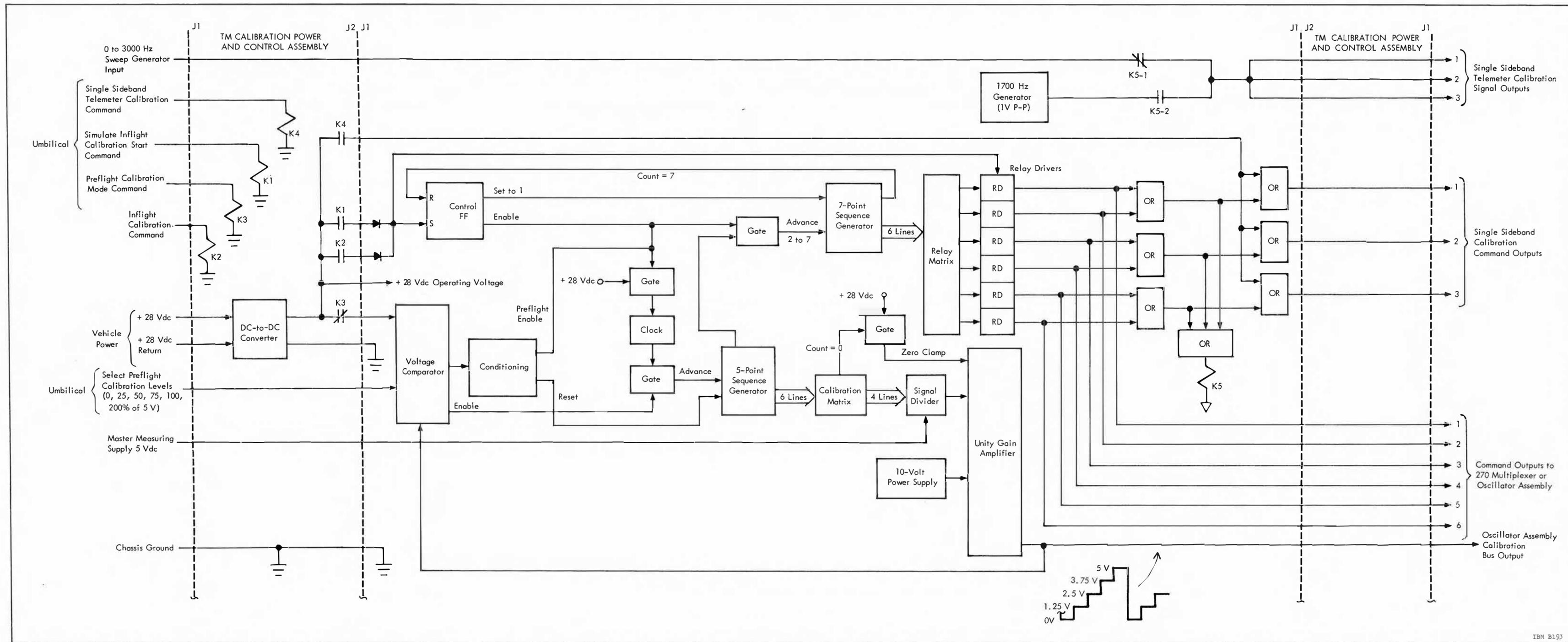
Figure 5.6-2 Telemetry Calibrator Assembly
