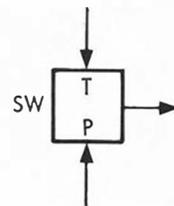
Bistable electronic switch (such as a silicon controlled switch). Input P is the "plate" or anode, and is connected to some power source. When P is present and trigger T occurs, the switch is said to be "on" and the output is then significant. Switch can be turned off only by an interruption of the power.
