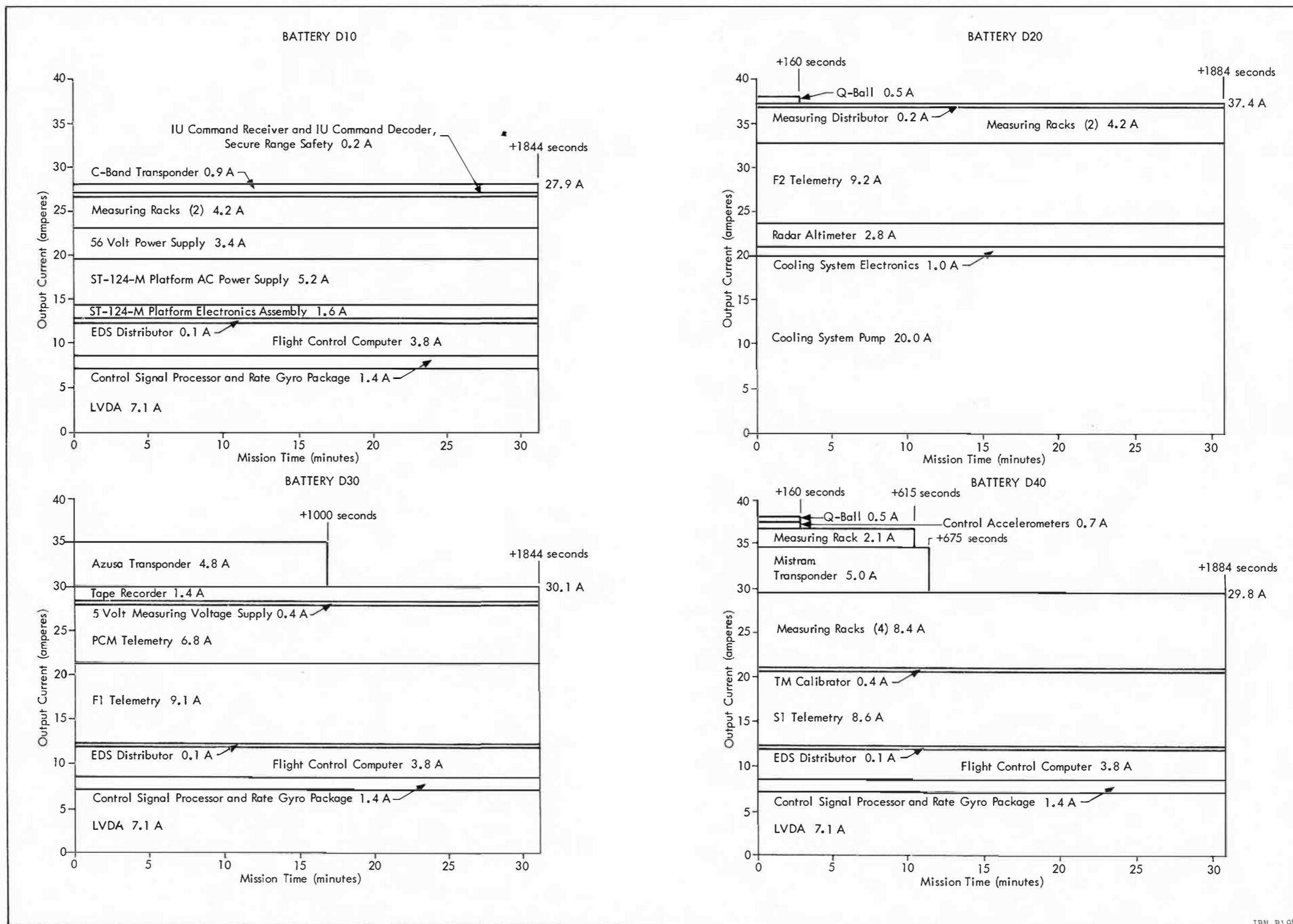
Figure 8.2-1 Battery Load Profiles for SA-IU-201
