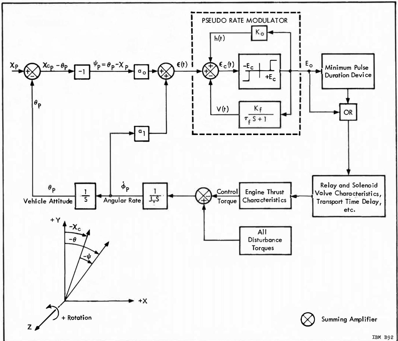
Figure 3.2-3 Pitch Channel of the Auxiliary Propulsion System
