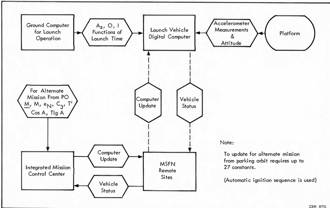
Figure 2.3-5 Linkage Between Vehicle and Ground
