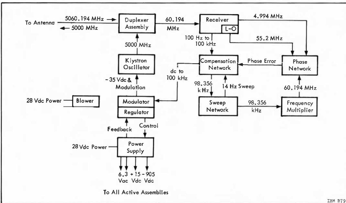
Figure 7.3-3 AZUSA Transponder Block Diagram
