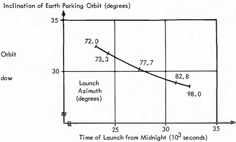
Time of Launch Versus Descending Node for a Typical Launch Window
