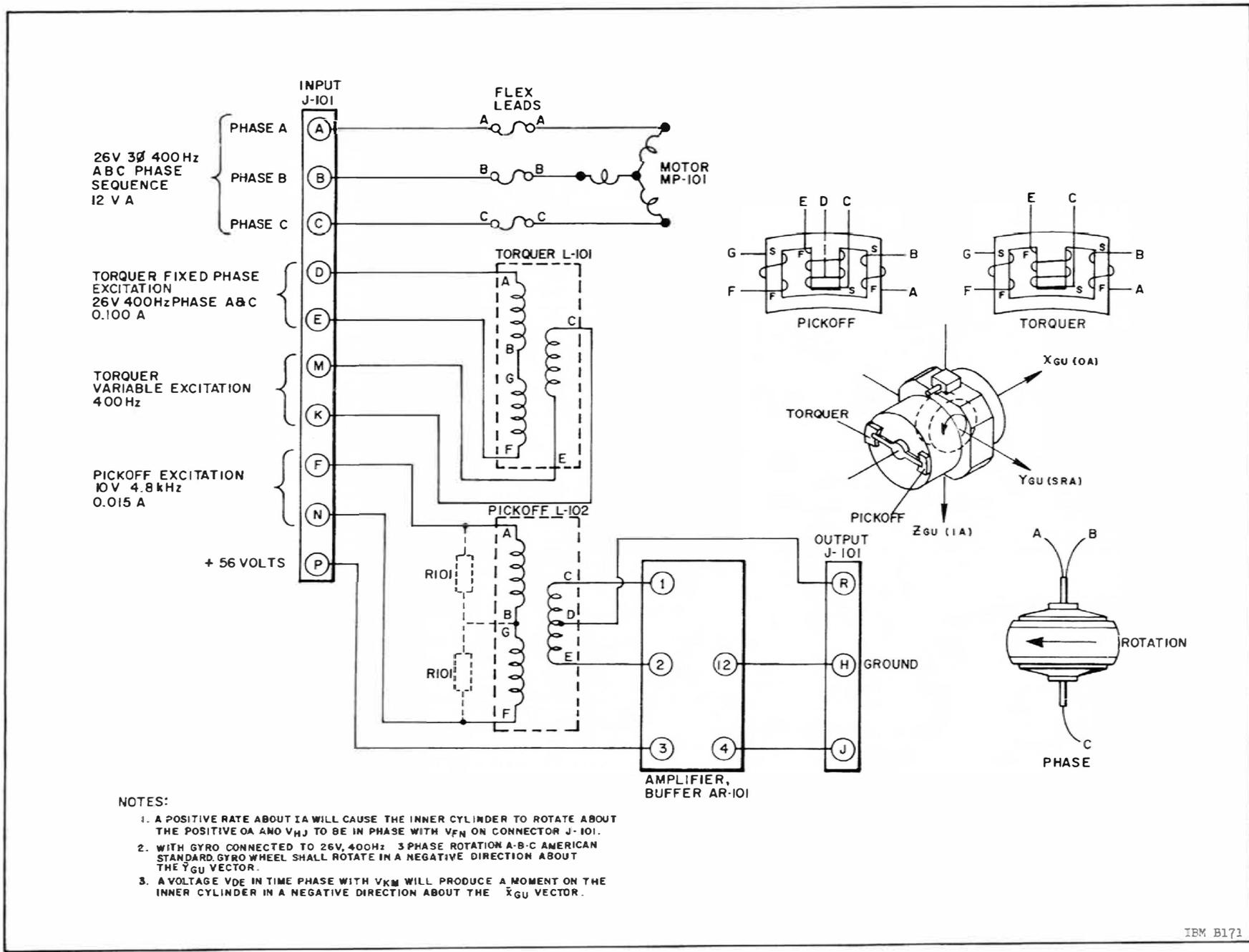
Figure 14.8-3 Electrical Schematic of an AB5-K8 Stabilizing Gyroscope
