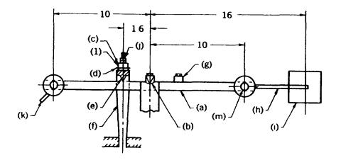
Deflection lever ratio of machine is 16 to 1.6
