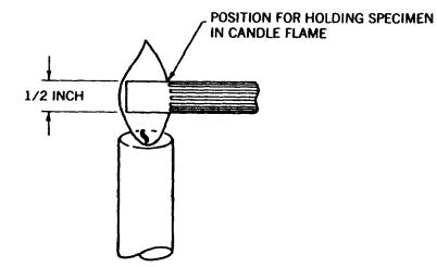
FIGURE 2. Flame-resistance test setup.
