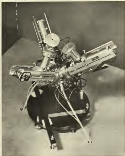
FIG. 1. AIR-BEARING MODEL OF THE FREE-ROTOR GYRO. (The rotor diameter is 2 in. Other sizes may be judged by the 6-in. ruler on the base plate.) The three optical sensors are located on the upper three faces of the cube which constitutes the gyro case.
