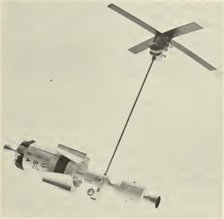
FIGURE 5. ATM TETHERED CONFIGURATION.
