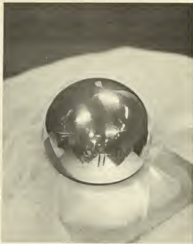
FIG. 2. AIR-BEARING GYRO ROTOR. The solid beryllium-copper rotor has been precisely machined to a 2-in. diameter. Sphericity is better than 25 \mu\text{in} . Clearly visible are the D-pattern, the dentate equatorial pattern, and the marking modification of the dentate pattern to enable rotor phase to be determined. Note that the double-tooth phase marking lines up with the edge of the D.
