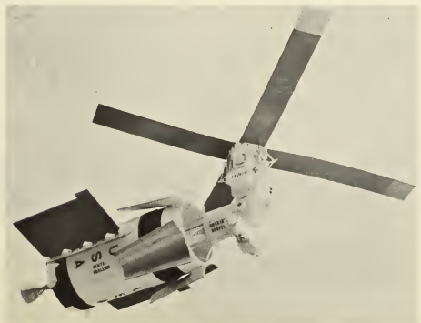
FIGURE 12. ATM STORAGE MODE CONFIGURATION.
