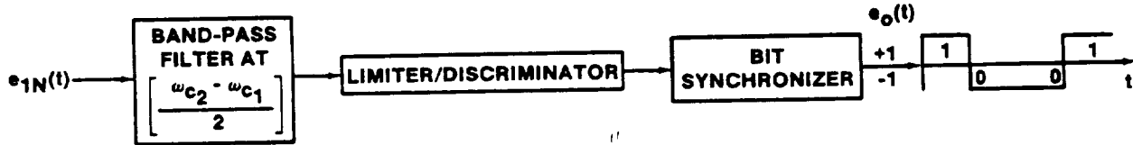
FIGURE 21.- SHUTTLE DIGITAL FM LINK DETECTION PROCESS.
