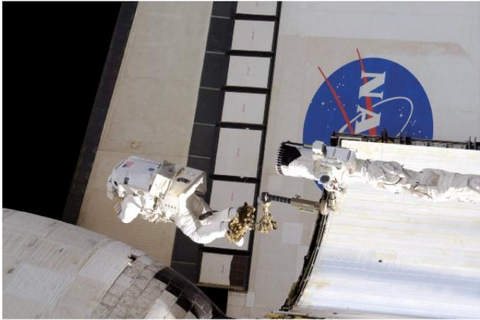
iss015e12948 -- EVA Repair: Anchored to a foot restraint on the RMS robotic arm, astronaut John "Danny" Olivas moves toward port OMS pod thermal blanket damage during EVA 3. Skin stapler and pins were used to make the repair.
