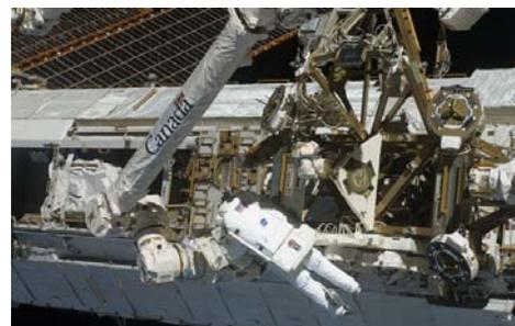
ISS021-E-030165 (19 Nov. 2009) Foreman installing a spare S-band antenna structural assembly to the Z1 segment of the station's truss. EVA 1.
