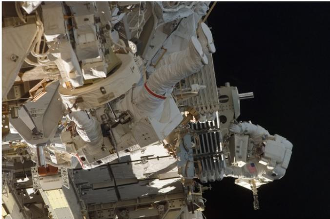
S117-E-06886 --- Reilly/EV1(center) Olivas/EV2 (right) connect power, data & cooling cables to S1 & S3, and deploy solar array blanket boxes on S4.
