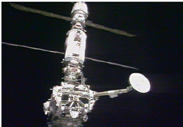
JSC2000-E-26636--- ISS after installation of Z1 Truss. From the top, elements are the Zvezda, the FGB or Zarya, Node 1 or Unity, and Z1.
