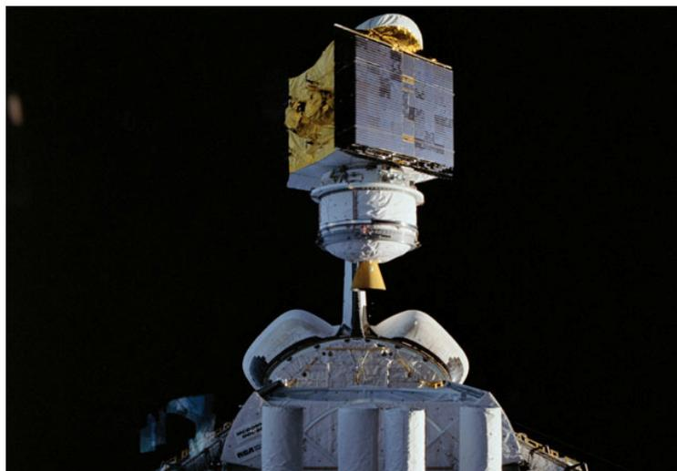
ABOVE: 61C-005-0036 -- SATCOM Ku-1 Communications Satellite deployed from Columbia.
