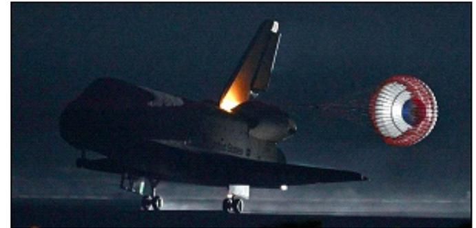
ABOVE: STS134-070 (1 June 2011) --- After 19 years of service, xenon lights illuminate Endeavour's drag chute during it's last landing & Shuttle's last night landing.
