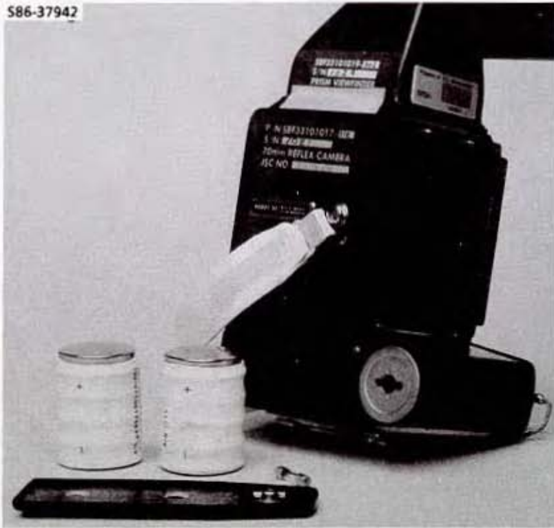
FUSE AND BATTERY LOCATION
