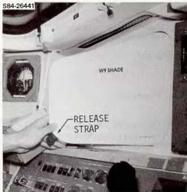
W9 SHADE INSTALLATION/REMOVAL
