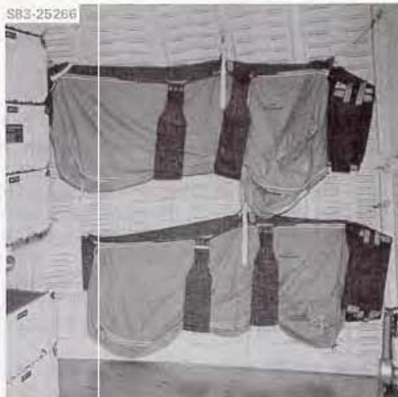
SLEEPING BAGS ON STARBOARD WALL- WHEN 4-TIER BUNK SLEEP STATIONS NOT FLOWN
