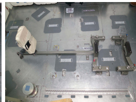
⑨ Install seat onto seat stem
