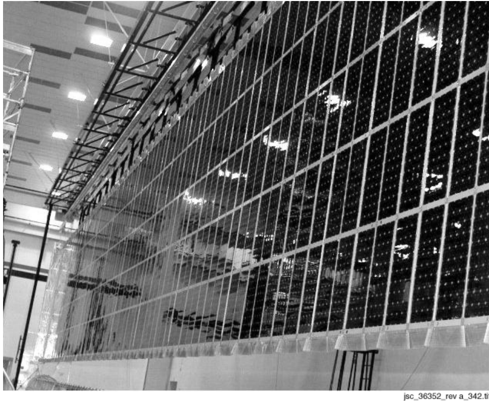
Figure 2-10. PV blanket (fully deployed)
