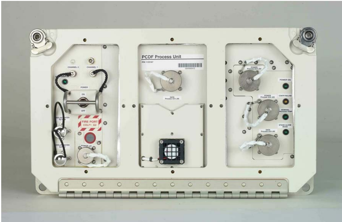
Figure 3-59. PCDF-PU front view after installation into MDL
