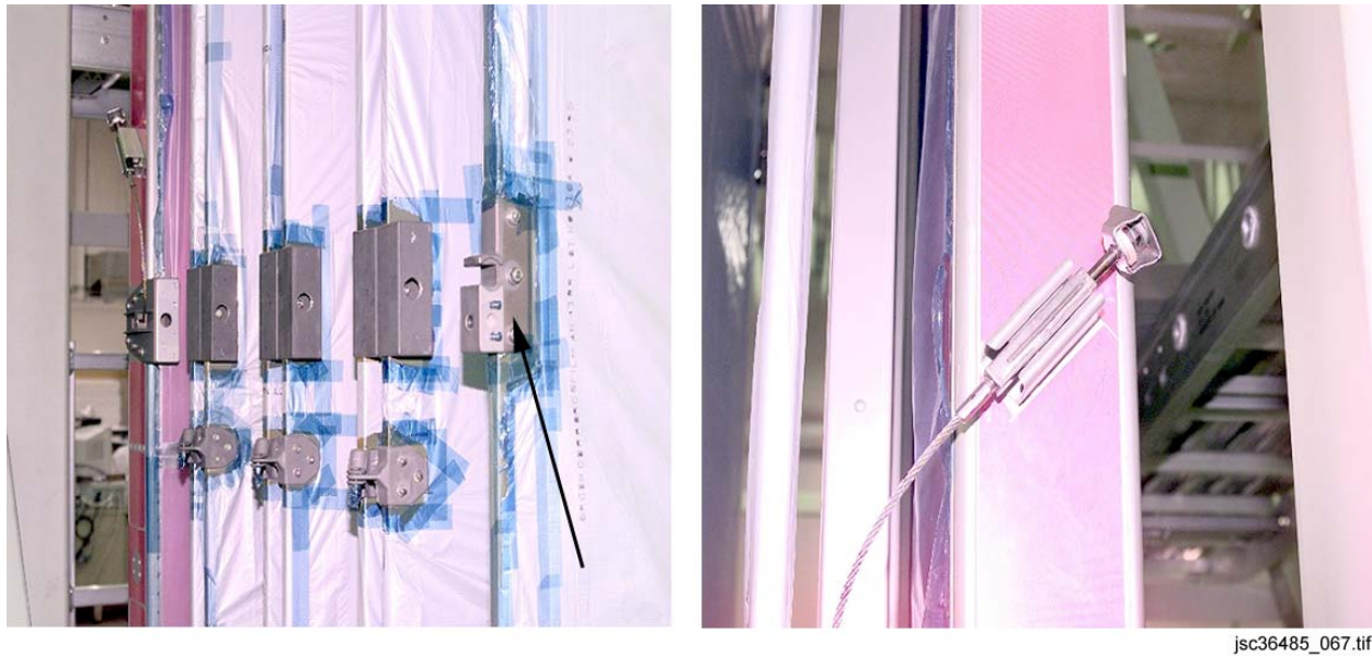
Figure 3-22. PVR cinch (left view – cinch receptacle; right view – secured in the on-orbit clip)
