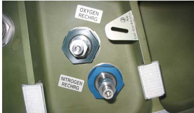
Figure 4.- MLI Velcro and PTCS Interfaces on NOD2 Bulkhead (MLI removed).
