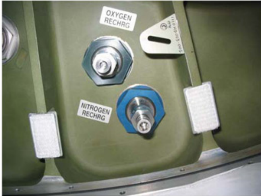
Figure 7. MLI and PTCS Interfaces on NOD2 Bulkhead (MLI Removed).
