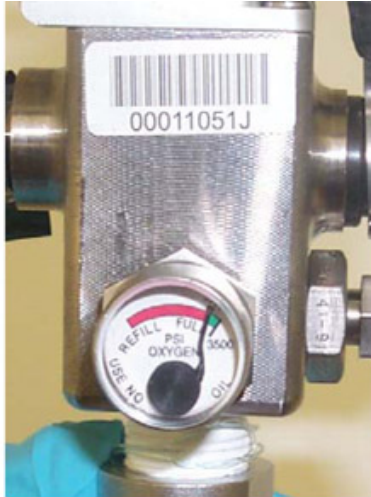
Figure 2-1 Acceptable Pressure Gauge Reading (Kapton Tape not shown)
