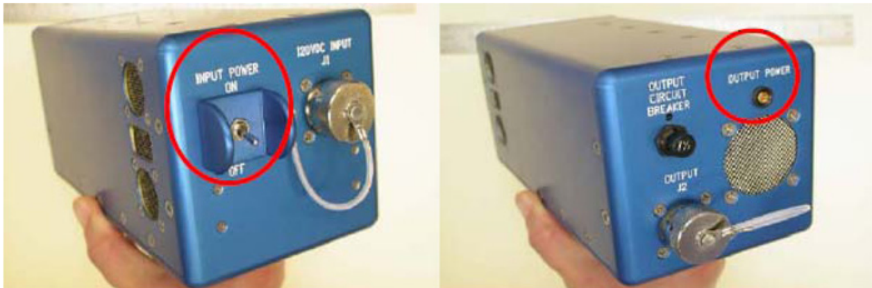
Figure 1. USOS A31p120V DC Power Supply Input Side with Power Switch on Left, Output Side with Output Power Light on Right.
