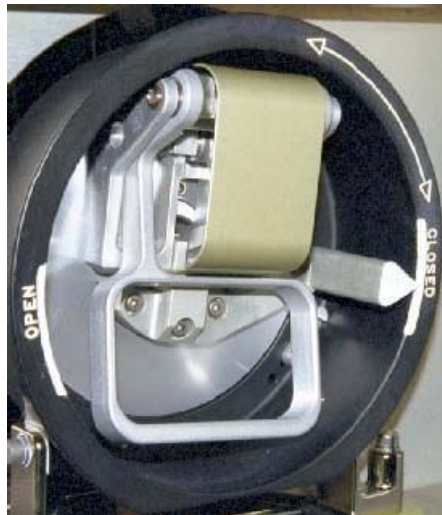
Figure 11.- Remote Manual Operator (RMO) with Indicator in Closed Position.
