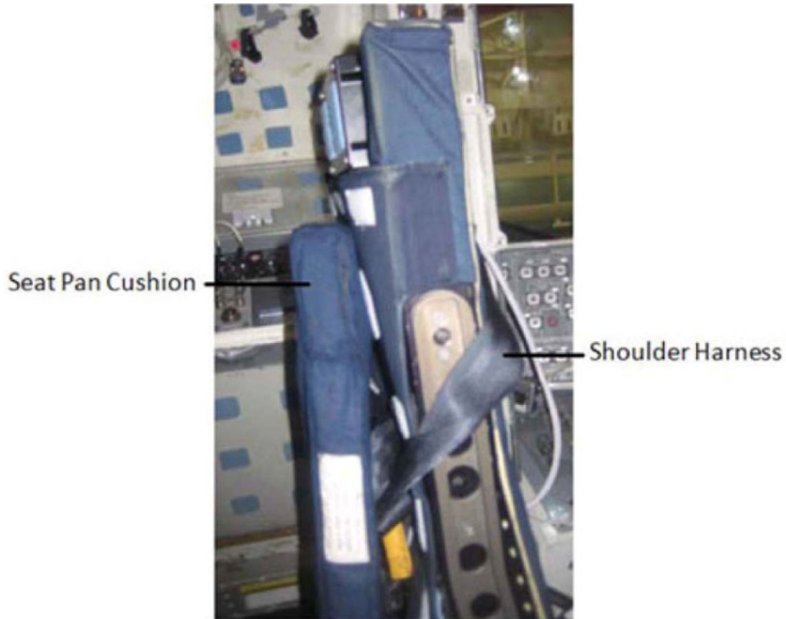
Figure 1. Shoulder Harness Wrapped Around CDR Seat Back.
