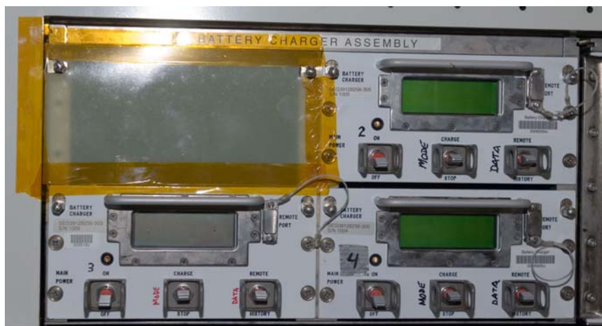
Figure 8.- FDF Cover for BCM-1 Opening.
