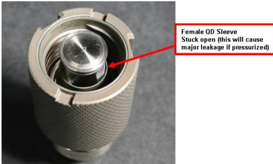
Figure 4. Large Female QD (Parker) with sleeve stuck in open position
