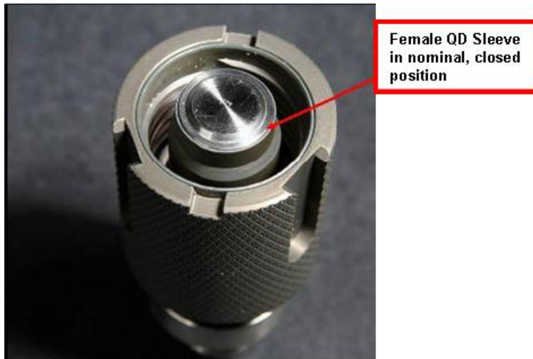
Figure 3. Large Female QD (Parker) with sleeve in nominal position
