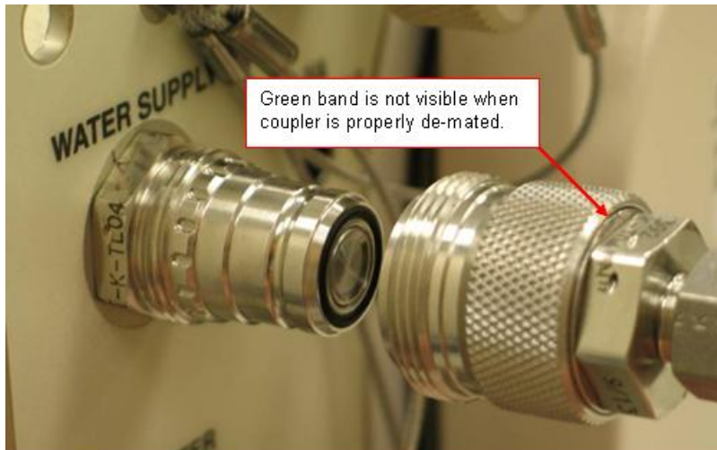
Figure 5. Properly de-mated small QD coupler.
