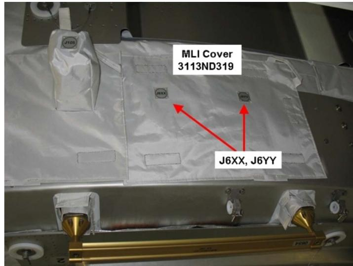
**Figure 3-5. LTA heater connectors MLI cover**
