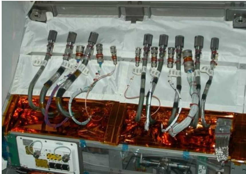
Figure 1.- NOD3D5, WRS-1 Umbilicals in Launch Restraints.
