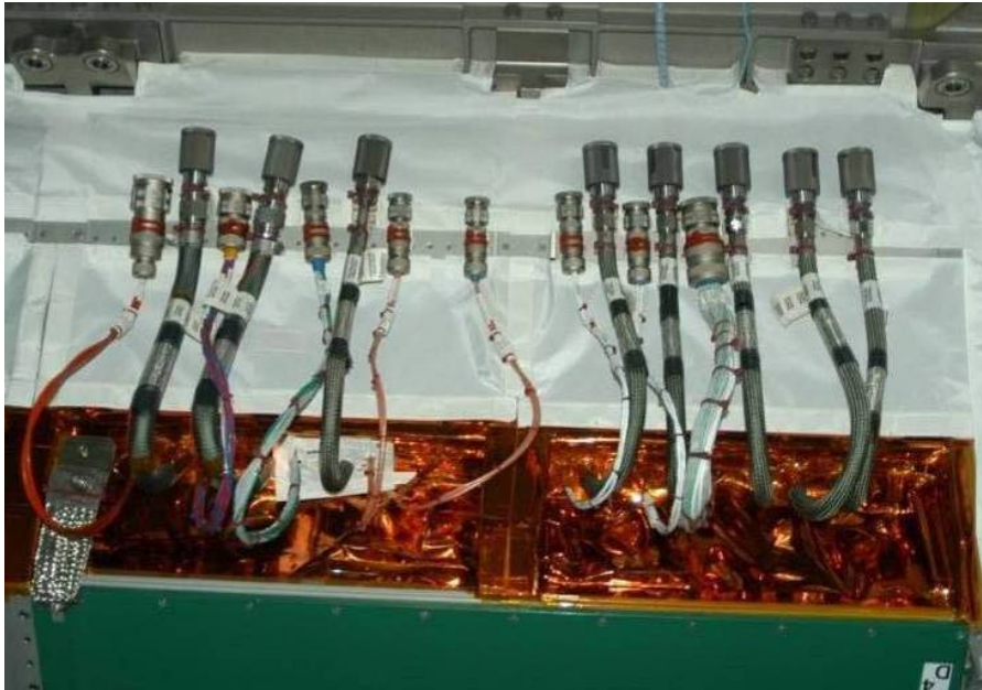
Figure 2.- NOD3D4, WRS-2 Umbilicals in Launch Restraints.
