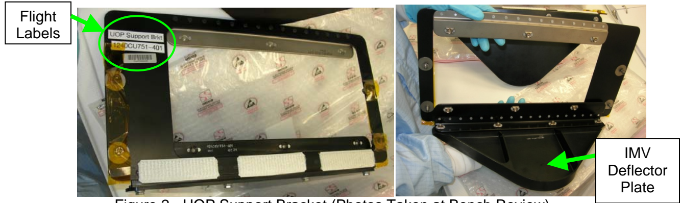
Figure 2.- UOP Support Bracket (Photos Taken at Bench Review).
