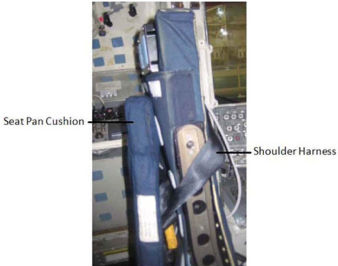
Figure 1. Shoulder Harness Wrapped Around CDR Seat Back
