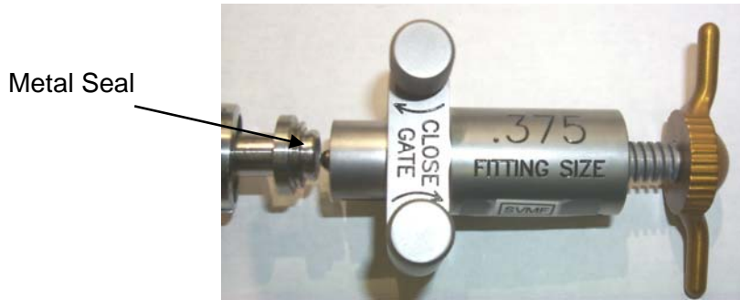
Figure 14.- Alignment of Gamah Seal Removal Tool and Gamah Fitting.
