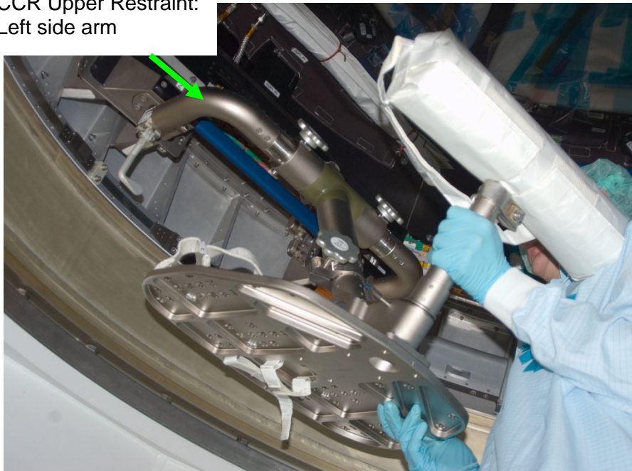
Figure 8. Cupola Crew Restraint – Installed.
