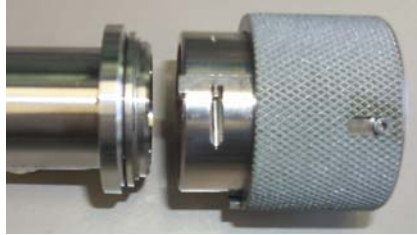
Figure 6.- Alignment of Ring Removal Tool and Gamah Fitting.
