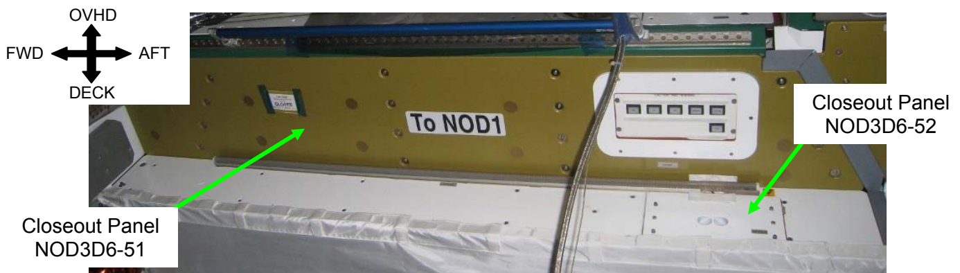
Figure 16.- Node 3 Starboard Endcone Deck Closeout Panels (looking Starboard).
