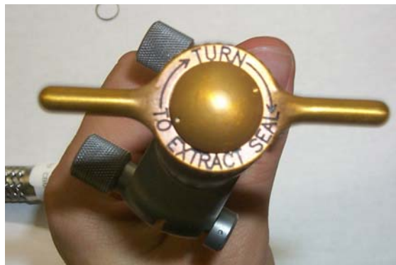
Figure 17.- Rotate Plunger Handle to Hardstop.
