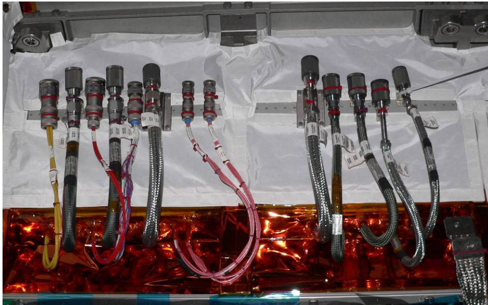
Figure 1.- NOD3A5 Umbilicals in Launch Restraint.
