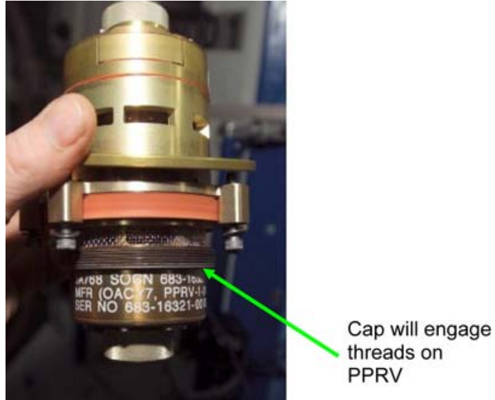
Figure 2.- PPRV Showing Threads for Cap.
