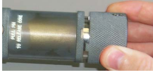
Figure 3.- Unscrew Ring Removal Tool Off of Ring Installation Tool.
