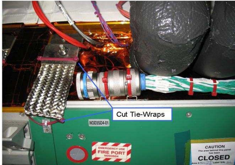
Figure 3.- ARS Ground Strap with Tie Wraps (Launch Configuration).
