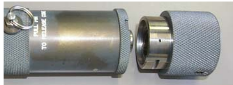
Figure 4.- Completely Disengage Ring Removal Tool from Ring Installation Tool.
