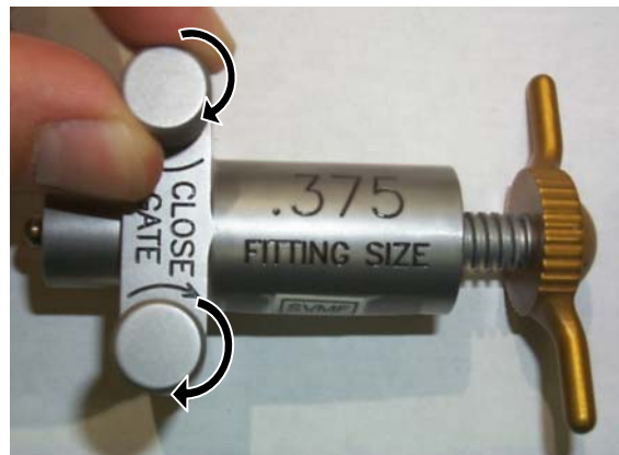
Figure 19.- Remove Tool from Gamah Fitting (Seal is Kept Inside Tool Barrel).
