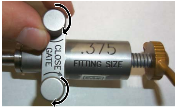
Figure 16.- Tighten Gate Knobs Until Gate is Clamped Onto Metal Seal.
