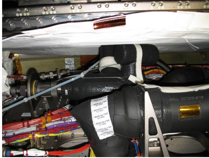
Figure 4.- NOD306 ITCS Coolant Sampling Adapter - Final Configuration.
