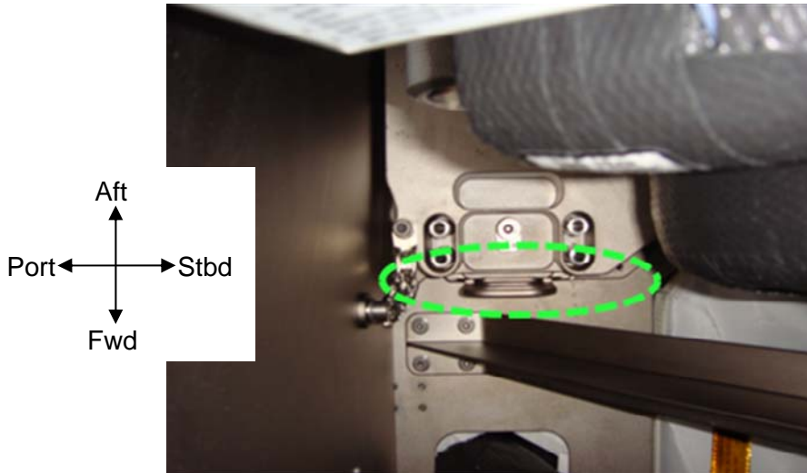
Figure 10.- U-Shaped AVM Blocking Device.
