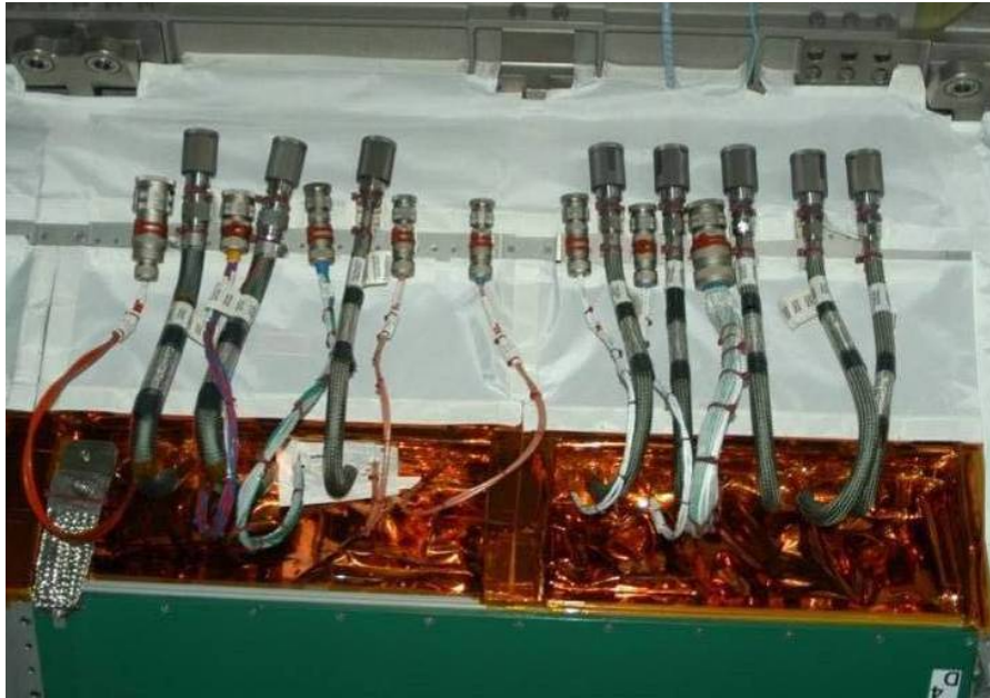
Figure 2.- NOD3D4, WRS-2 Umbilicals in Launch Restraints.
