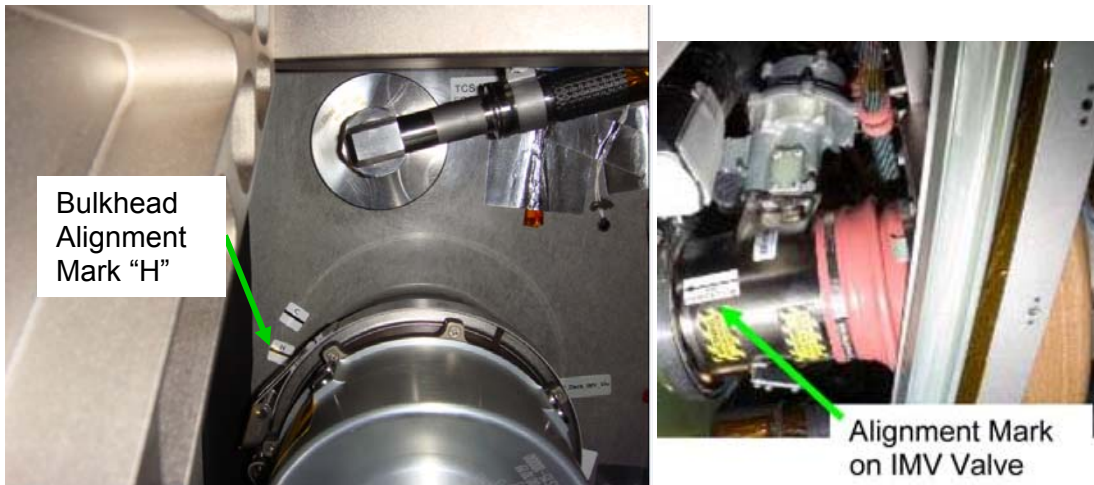
Figure 7. - Bulkhead Alignment Mark and IMV Valve With Alignment Mark.
