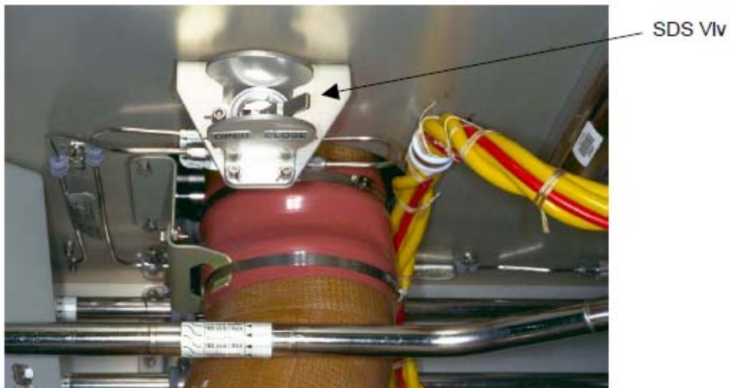
Figure 21.- NOD1 Deck Manual SDS Valve (Under NOD1D1-01 Closeout Panel).
