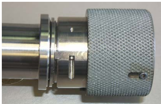
Figure 8.- Place Removal Tool onto Gamah Fitting.
