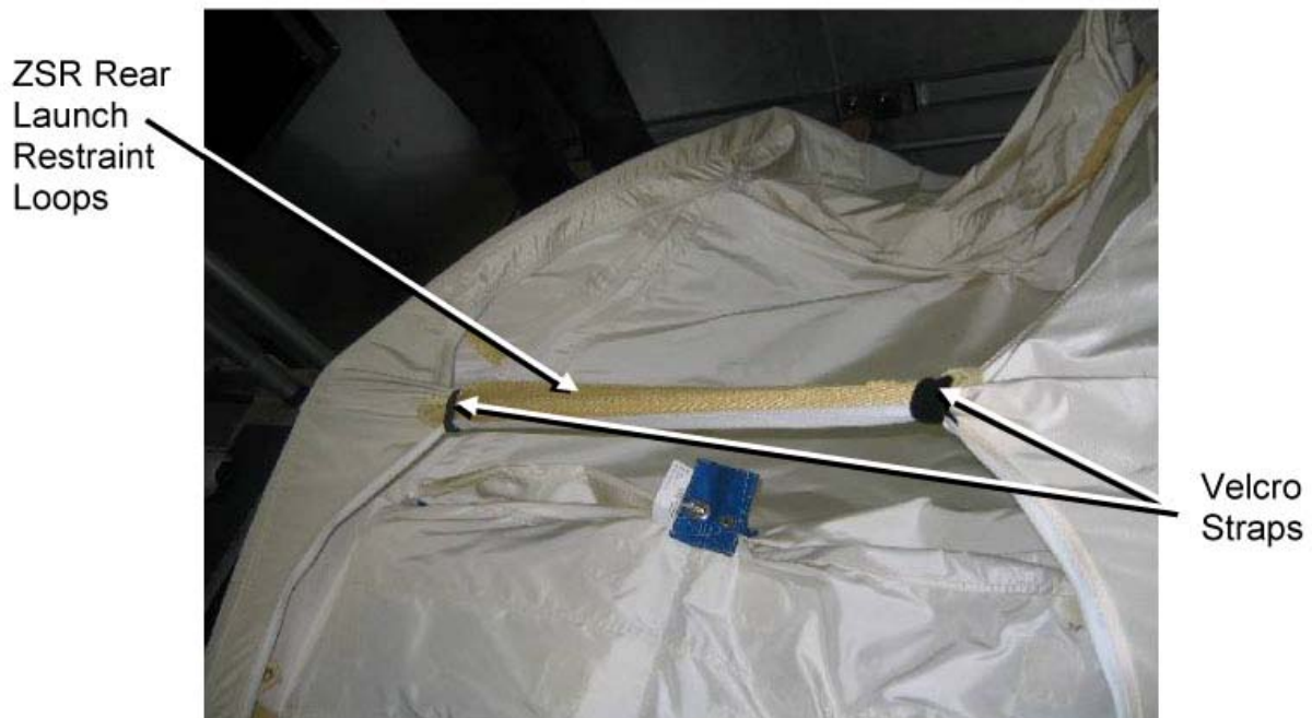
Figure 12.- ZSR Rear Launch Restraint Loops Restrained with Velcro Straps.
