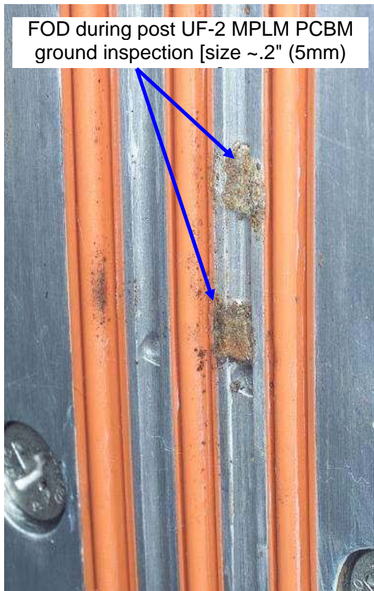
Figure 5.- FOD (Left) and Resulting Damage (Right) on MPLM PCBM Seals and Seal Substrate - FOD Occurred on Flight UF-2.
