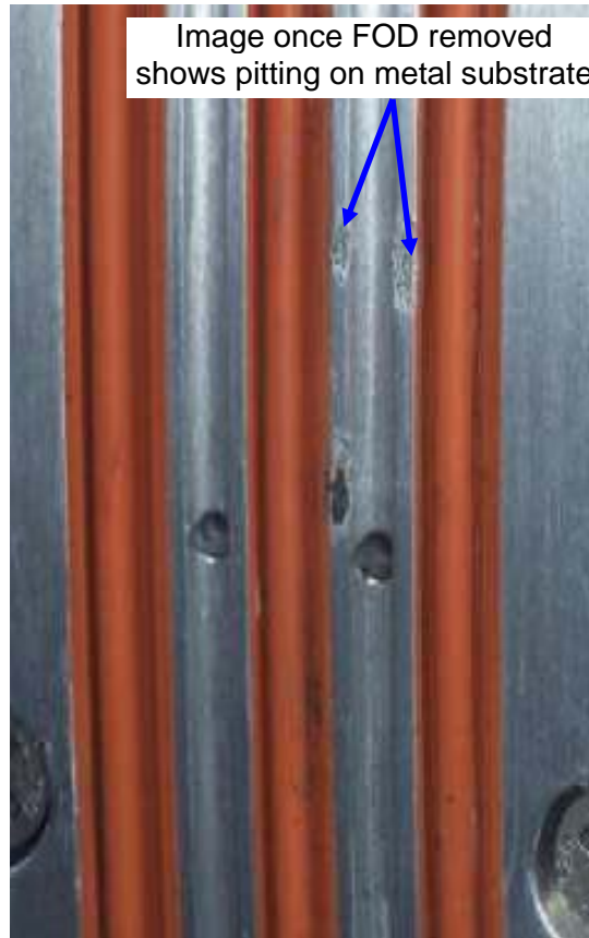
Figure 5.- FOD (Left) and Resulting Damage (Right) on MPLM PCBM Seals and Seal Substrate - FOD Occurred on Flight UF-2.
