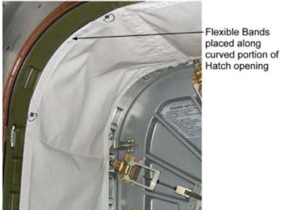
Figure 34.- Closeout Installed over Vestibule.
