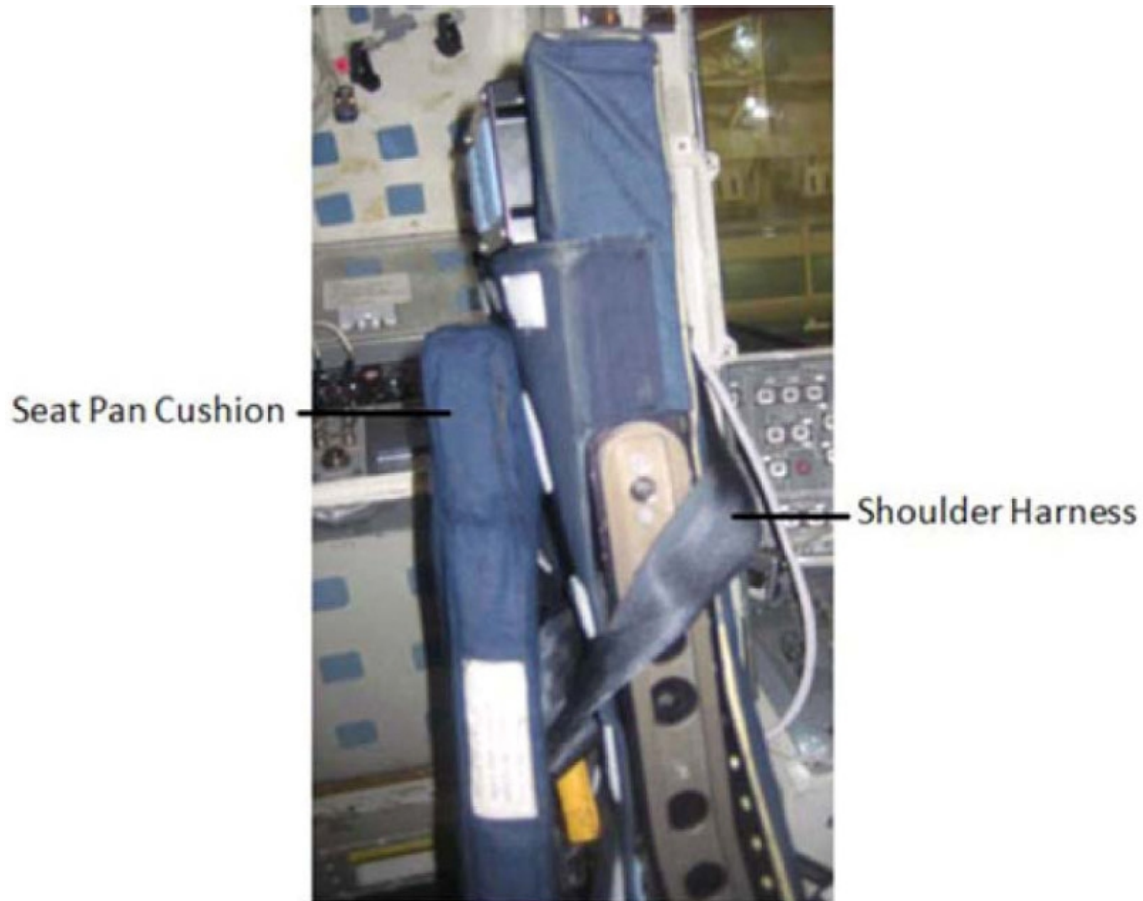
Figure 1. Shoulder Harness Wrapped Around CDR Seat Back
