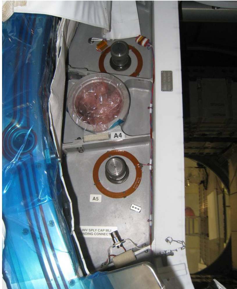
Figure 25.- PMM Bulkhead Feedthroughs - Aft Quadrant (Ground Photo)
