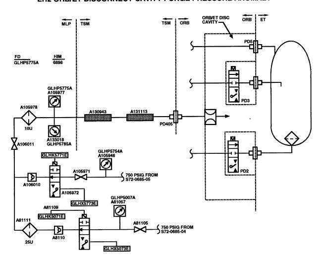
Figure 39-02 LH2 Orbiter/ET Disconnect Cavity Purge Pressure
