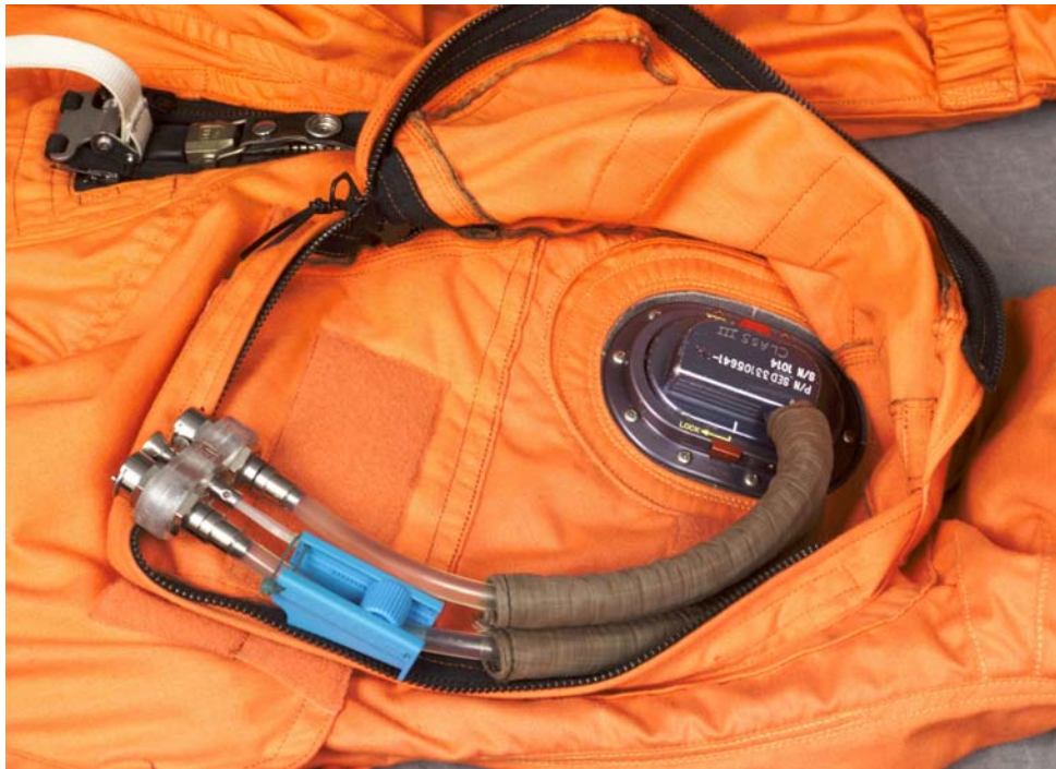
Figure 2-33. Liquid cooling BIP plug installed in suit
