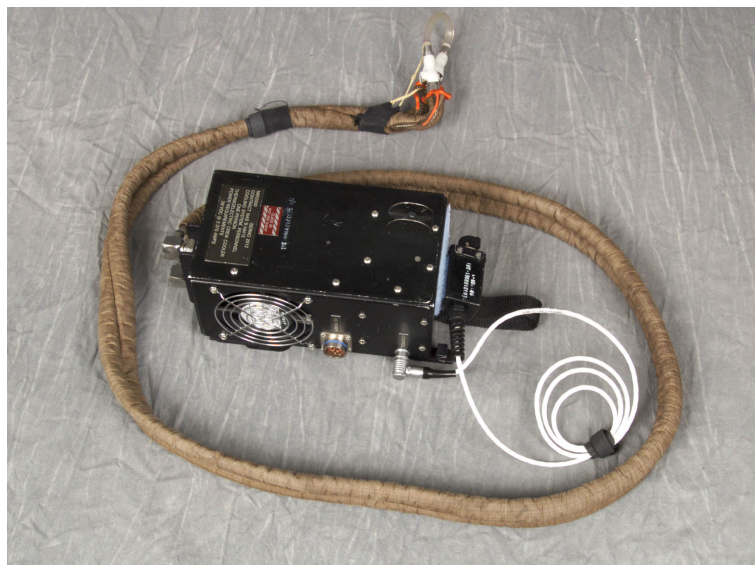
Figure 2-28. Individual Cooling Unit
