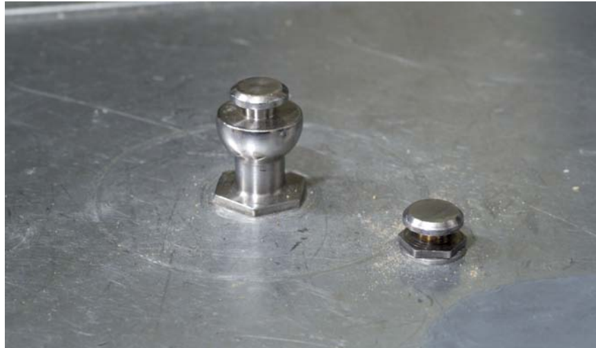
Figure 5-19. Seat deck studs
