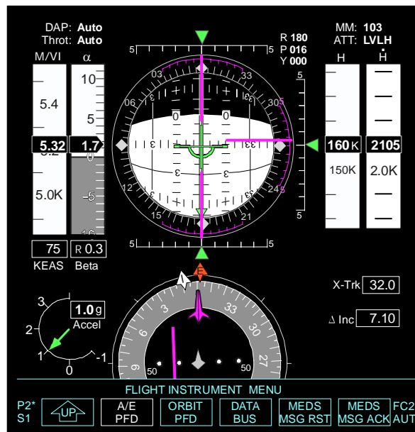
Figure 9-6. Example of Ascent/Entry PFD in MM 103
